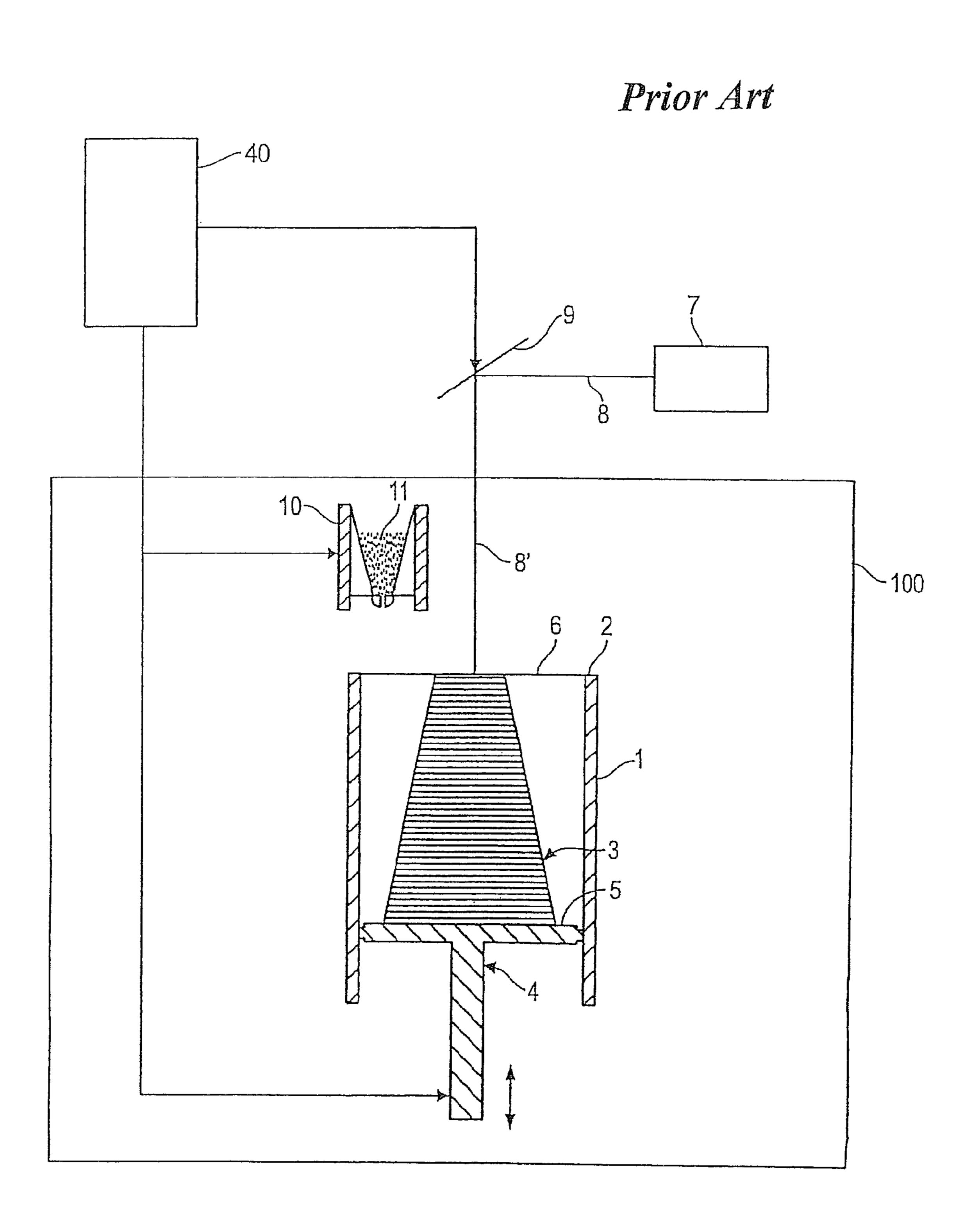
INFLUENCING SPECIFIC MECHANICAL PROPERTIES OF THREE-DIMENSIONAL **OBJECTS MANUFACTURED BY A** SELECTIVE SINTERING BY MEANS OF ELECTROMAGNETIC RADIATION FROM A POWDER COMPRISING AT LEAST ONE POLYMER OR COPOLYMER
