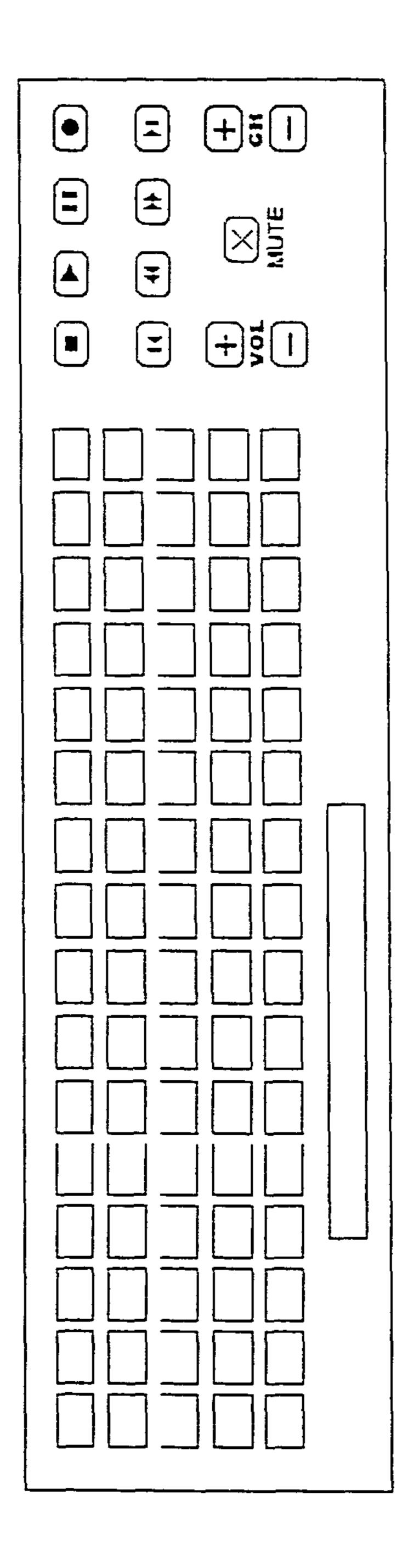
Figure 3. Standard Keyboard With Audio/Video Play Out Control Keys
