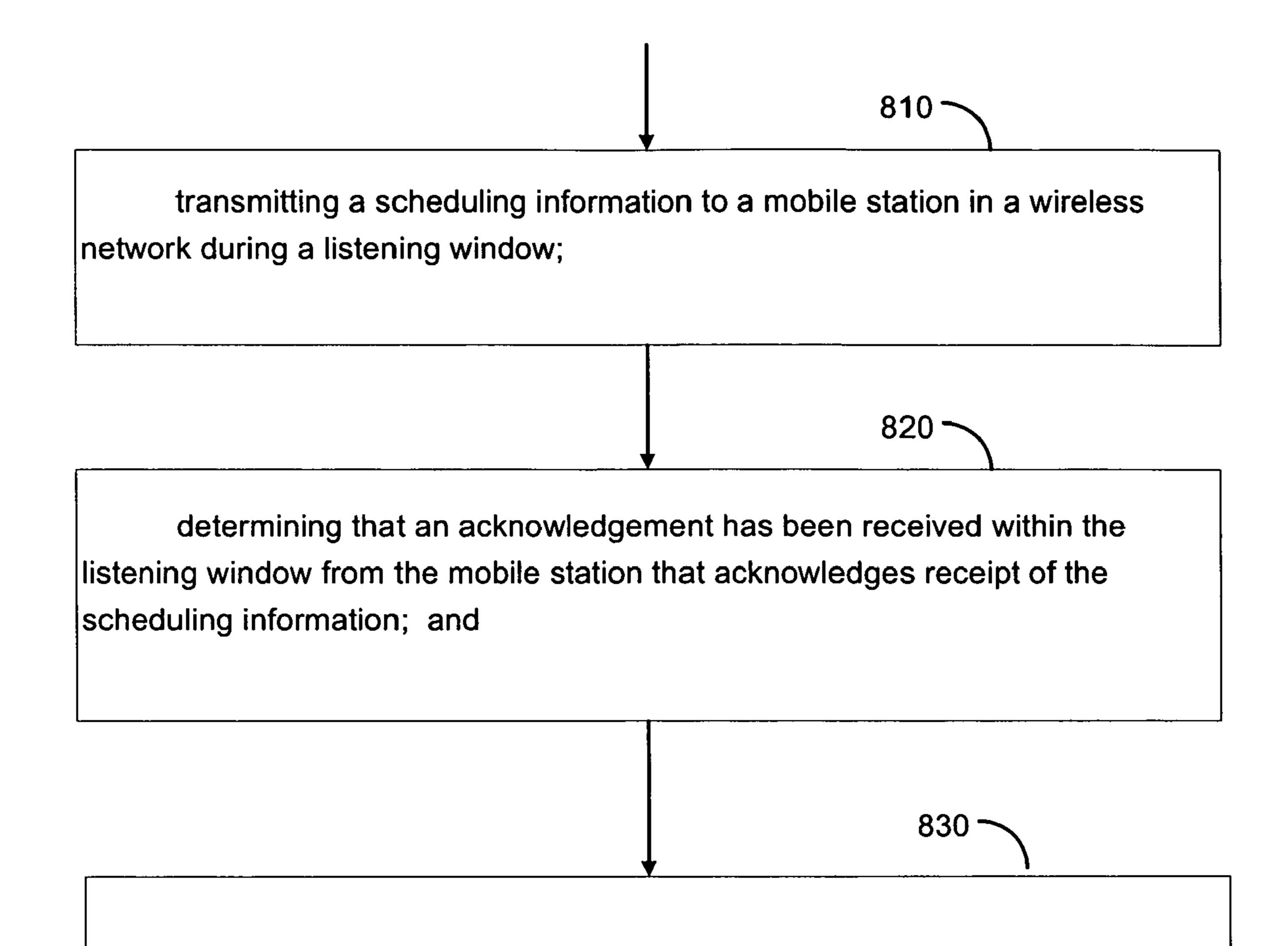
resetting a size of a next sleep window for the mobile station to an initial sleep window size based on the receipt of the acknowledgement.
