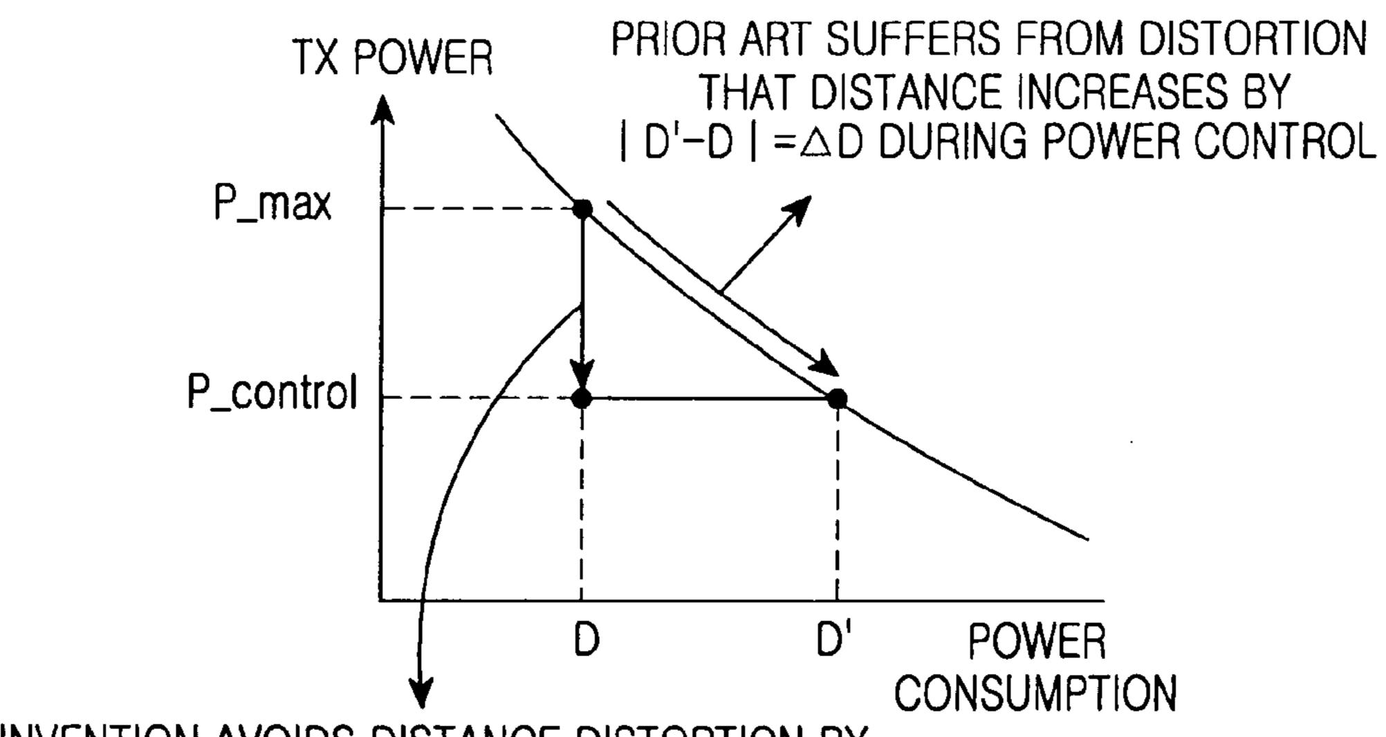
INVENTION AVOIDS DISTANCE DISTORTION BY SIMULTANEOUSLY PERFORMING MOBILITY ESTIMATION AND POWER CONTROL
