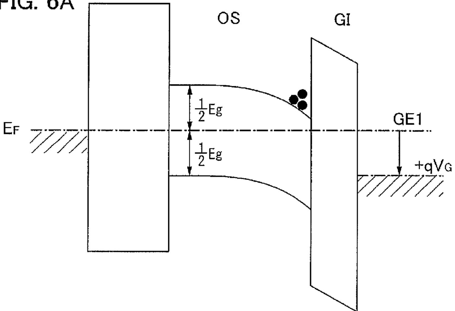
Energy band diagram of B-B' section ( $V_G > 0$ )
