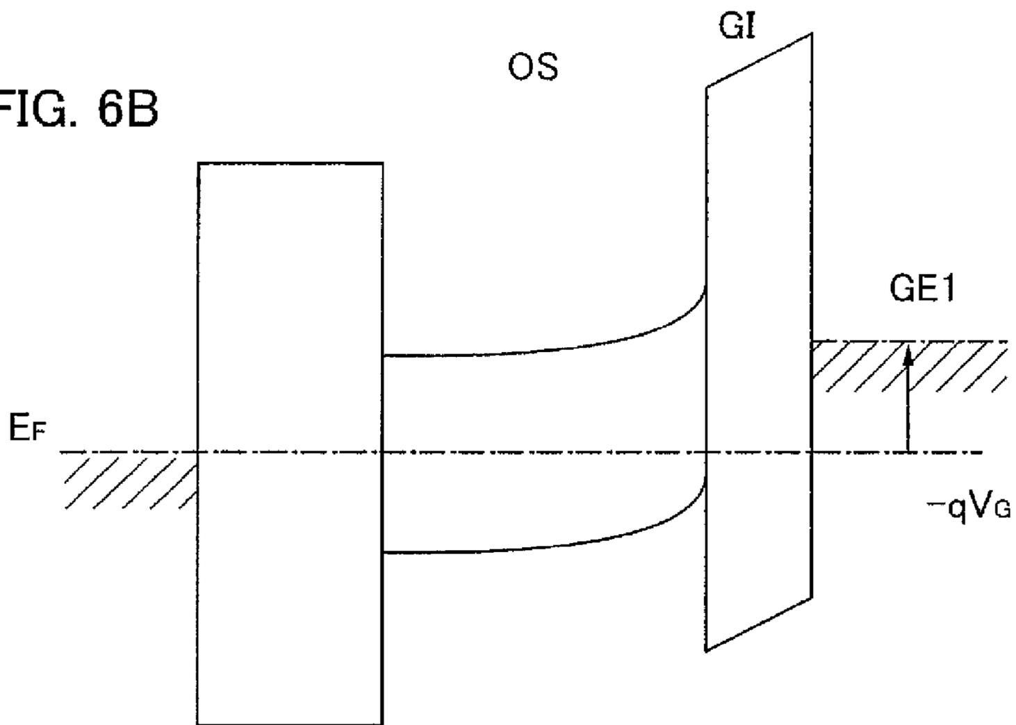
Energy band diagram of B-B' section ( $V_G < 0$ )
