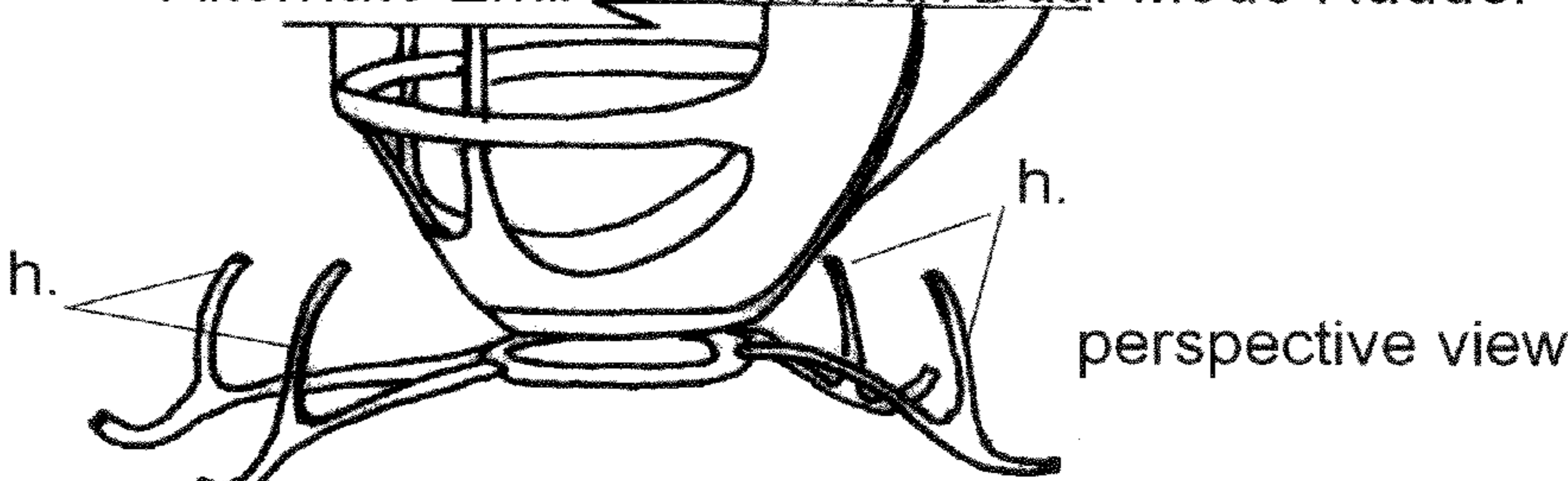
Fig. 20 AE Showing Four Upright Mounting Struts
