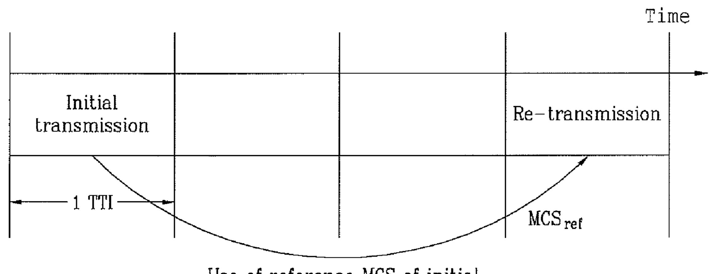
Use of reference MCS of initial transmission during re-transmission
