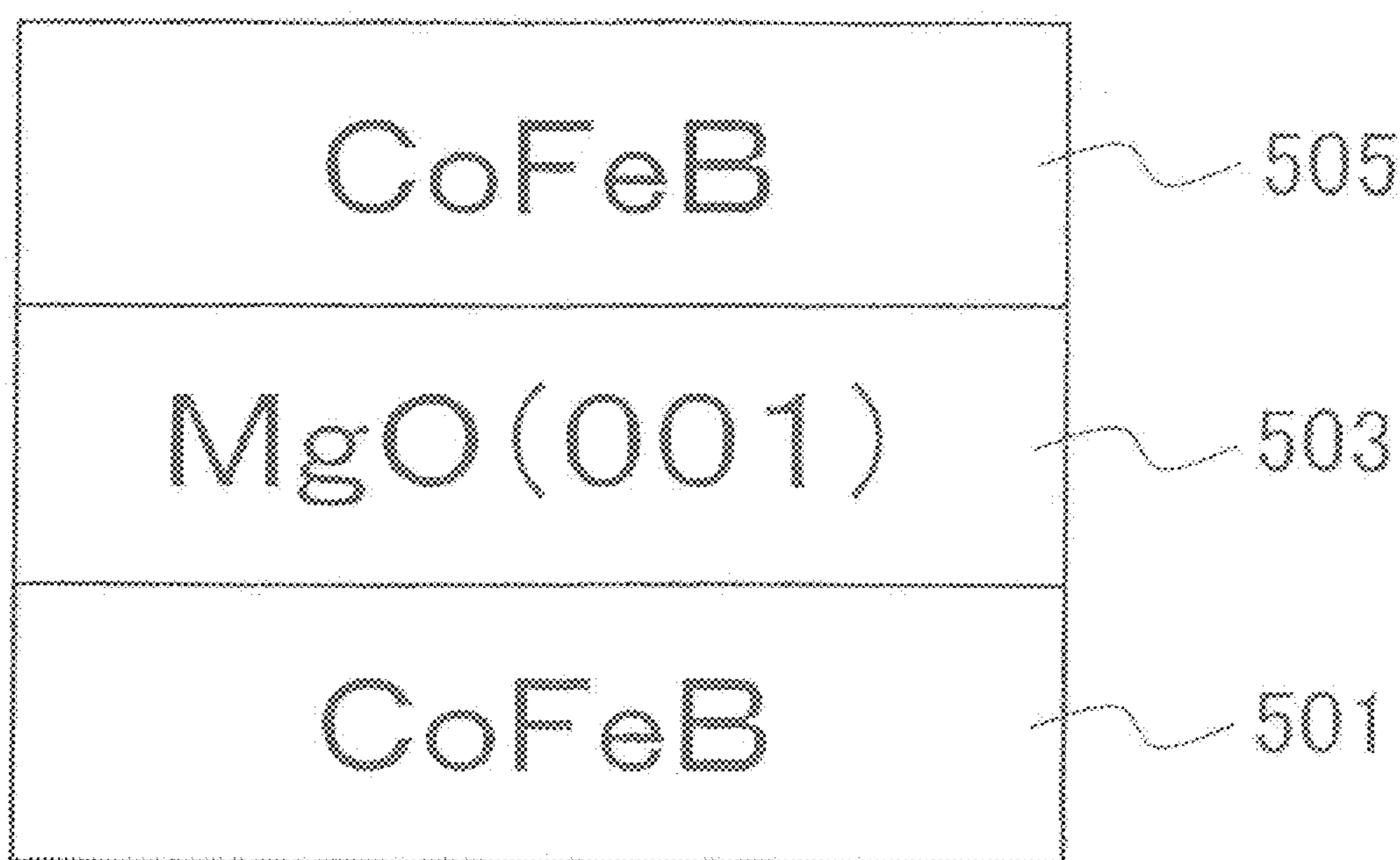
**MAGNETIC TUNNEL JUNCTION DEVICE****CROSS-REFERENCE TO RELATED APPLICATION**
