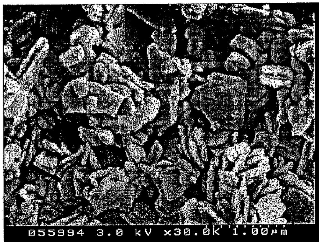
Scanning electron microscopy picture of BaClF:Sm<sup>3+</sup> as prepared according to Example 1 in the text.
