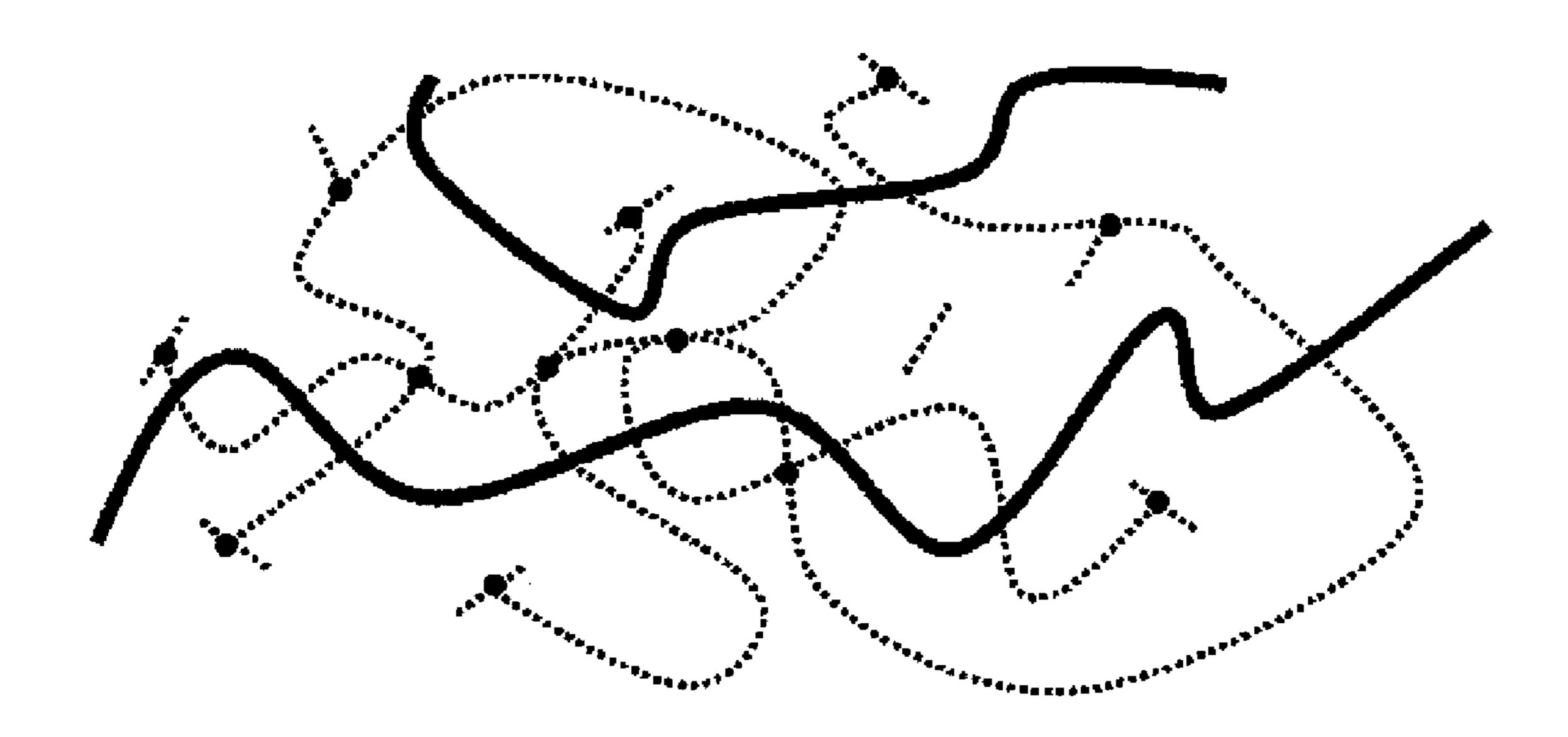
PROCESS FOR PRODUCING RESIN VARNISH CONTAINING SEMI-IPN COMPOSITE THERMOSETTING RESIN AND, PROVIDED USING THE SAME, RESIN VARNISH FOR PRINTED WIRING BOARD, PREPREG AND METAL-CLAD LAMINATE
