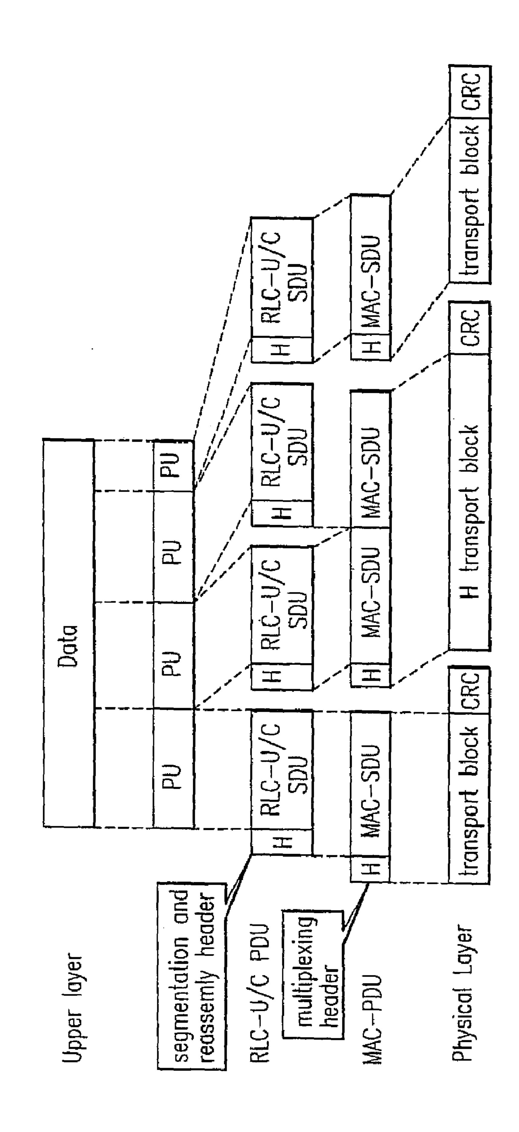
Data acknowledgment block header transport segmentation and reassembly header multiplexing header RLC-U/C PDU Physical Layer Upper layer MAC-PDU
