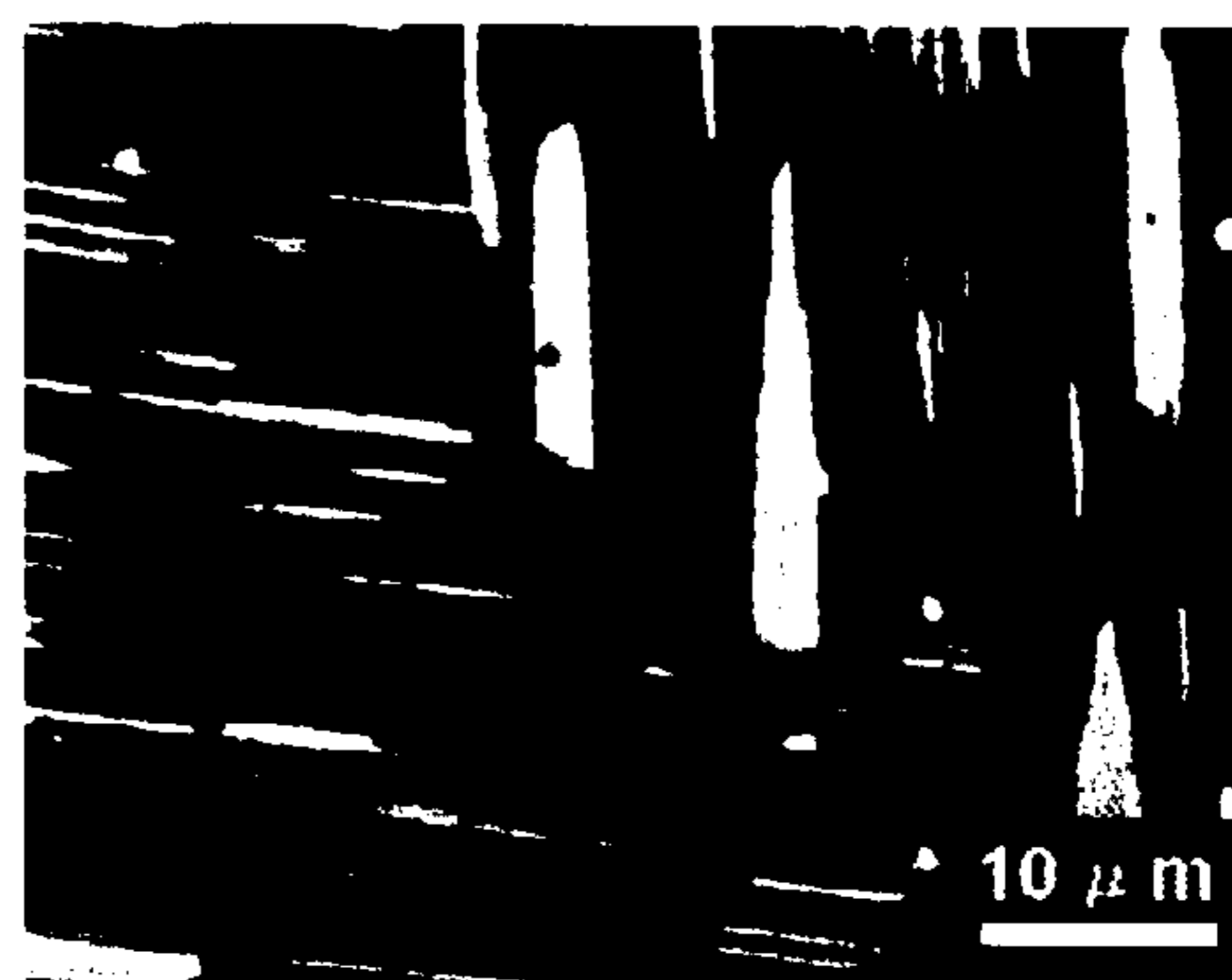
phase showing 14H-LPO + phase showing Mg_3Zn_3Gd_2
