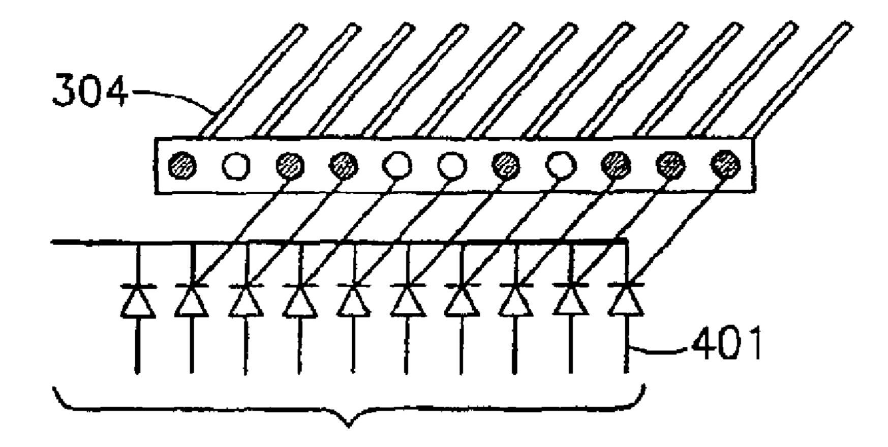
OUTPUT VECTOR TO DECIDE THE ROUTER SWITCHING POSITION AND DECIDE THE NEXT HOP ADDRESS ACCORDING TO ITS ROUTING TABLE
