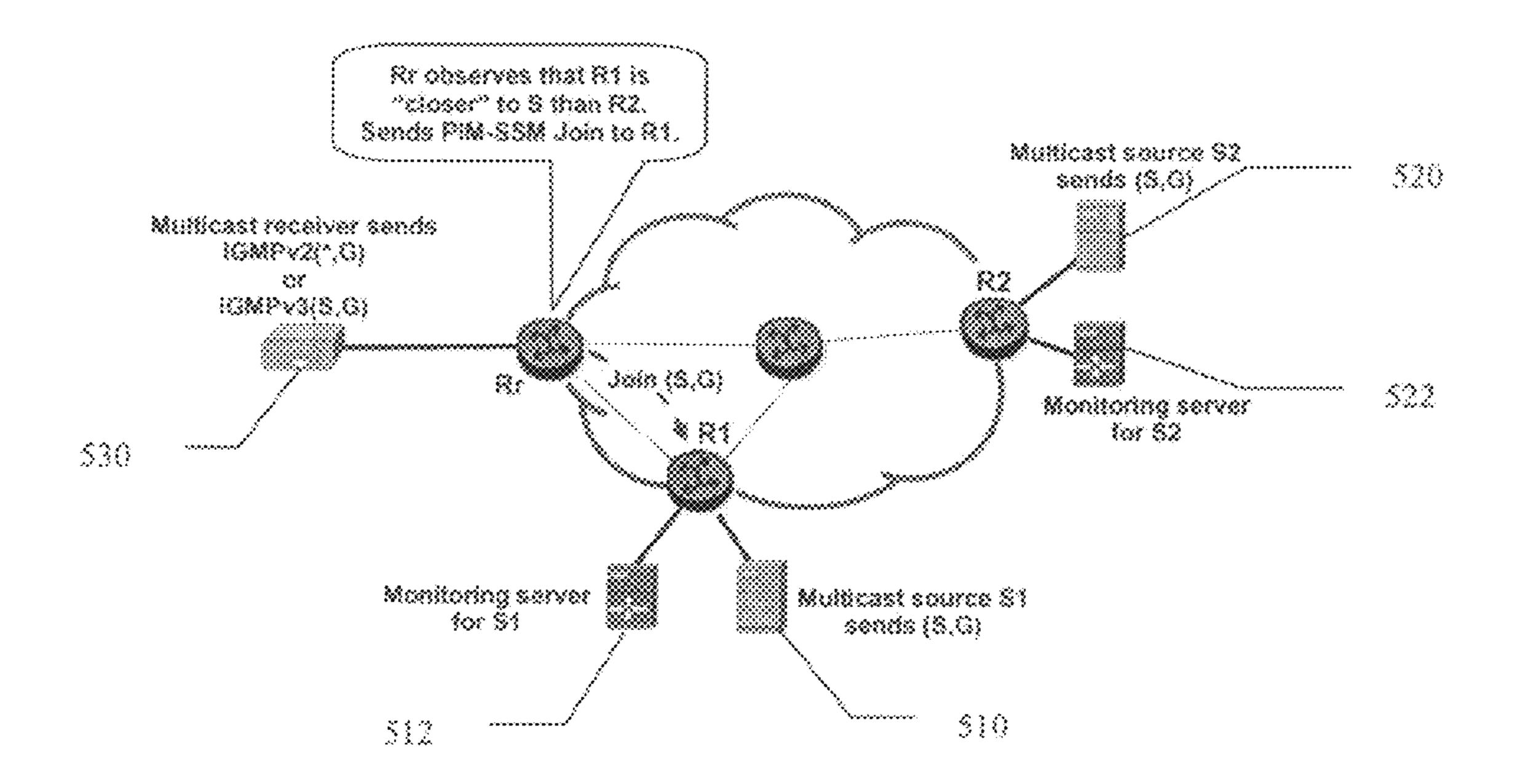
Figure 5 Example of Anycast Source operation
