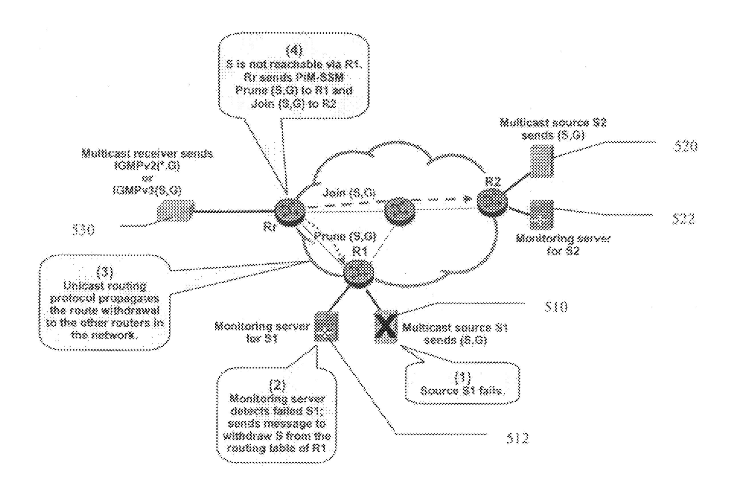
Figure 6 Example of automatic failuver operation when a source fails
