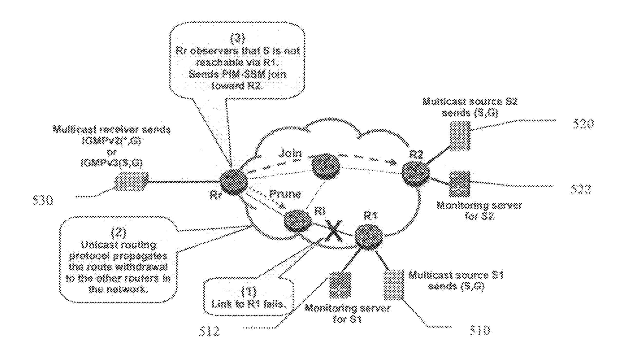
Figure 7 Example of automatic failurer operation after link failures
