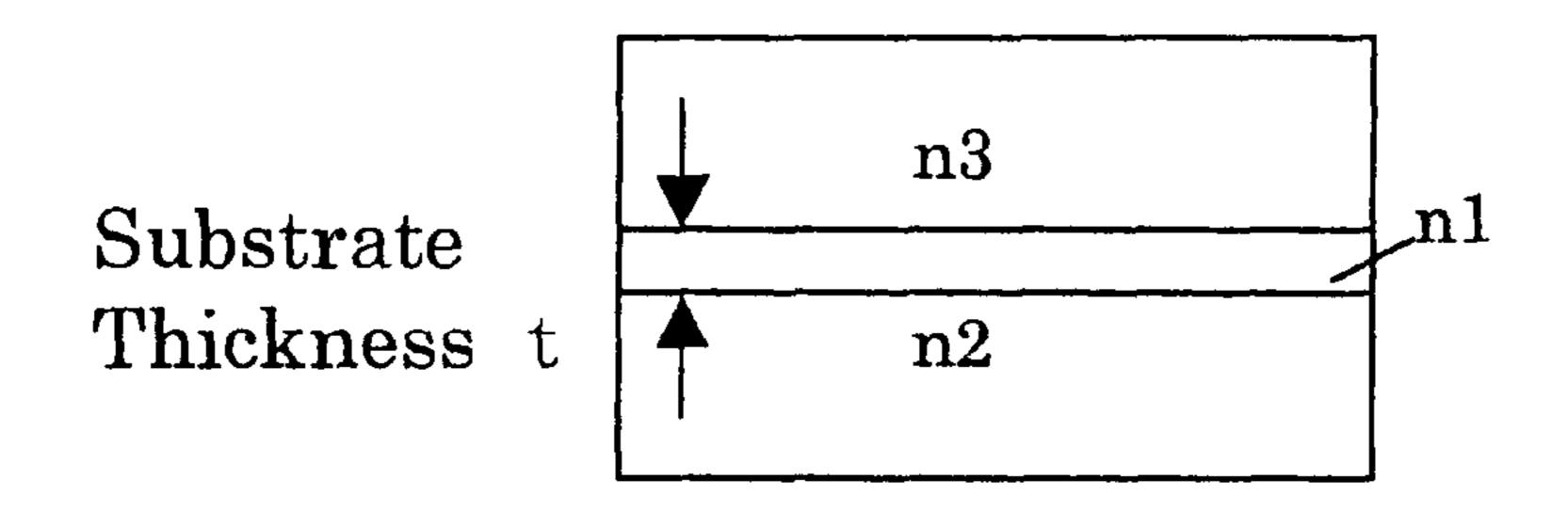
Calculating condition: n2, n3 are sufficiently thick
