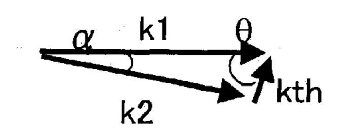
Parametric Wave oscillating condition (Cherenkov Radiation)
