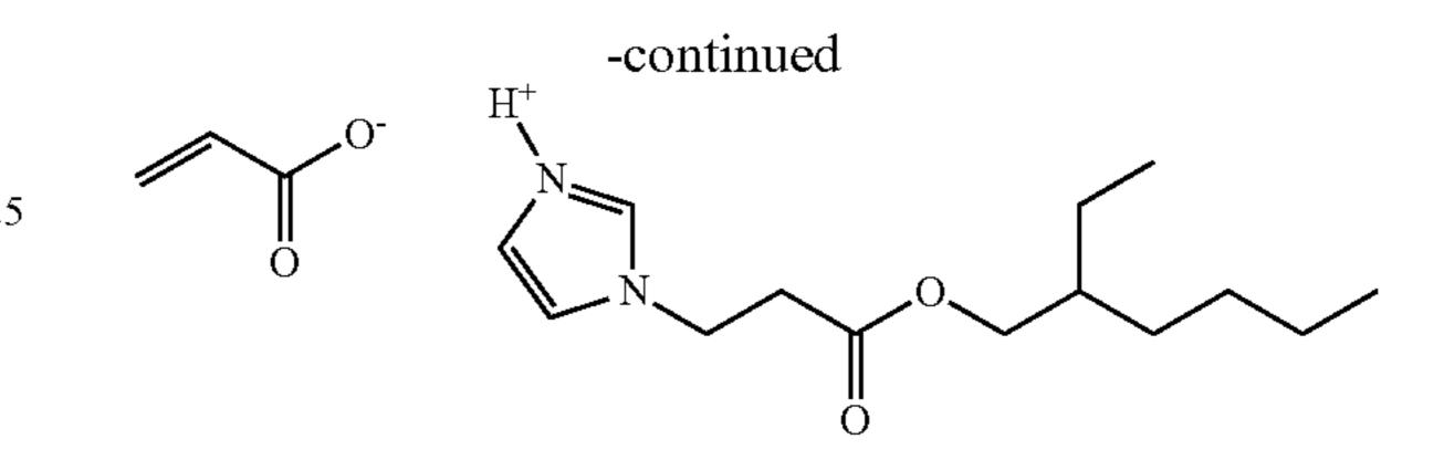
To an 8 oz. (236 mL) glass jar charged with 3-imidazol-1-yl-propionic acid 2-ethylhexyl ester (126.2 g, 0.50 mol, Preparatory Example 1) was added acrylic acid (36.0 g, 0.50 mol) and the jar was placed on a roller mill for 3 hours to mix. The product was a clear liquid.
