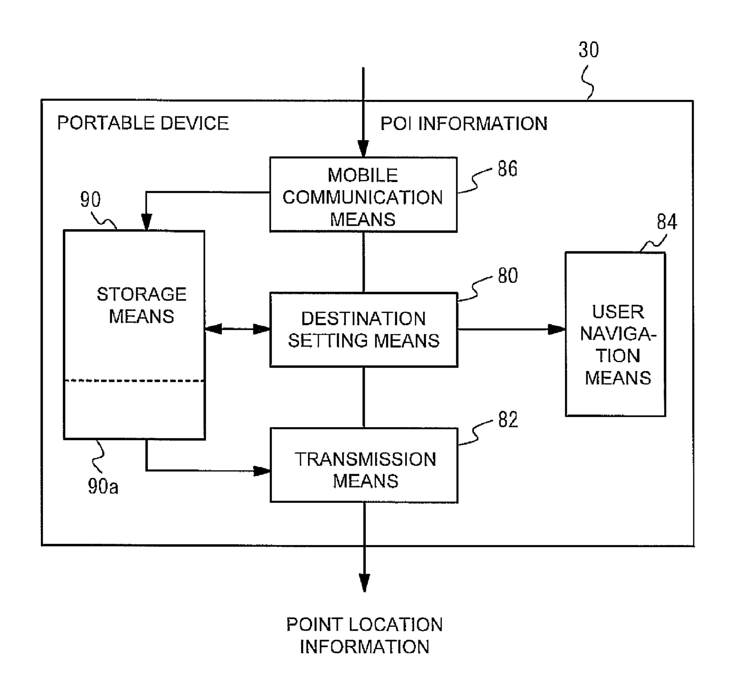
90a: STORAGE AREA FOR VEHICLE-MOUNTED DEVICE
