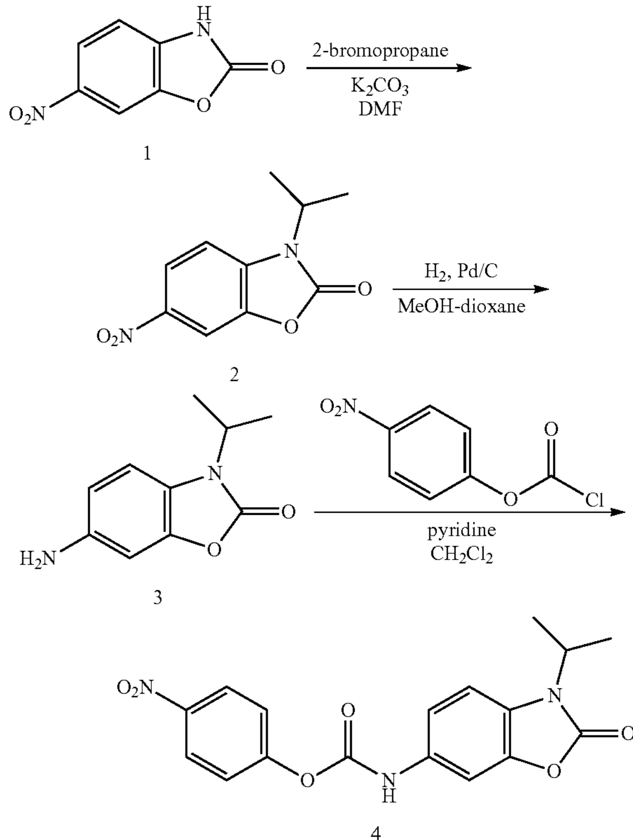
Commercial 6-Nitrobenzoxazole-2(3H)-one (Compound 1) (15 g, 83.28 mmol) was dissolved in DMF (200 mL), then to the reaction mixture, which was stirred at room temperature, were added potassium carbonate (23.02 g, 166 mmol)
