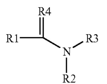
in which R1 is a hydrogen residue or a methyl residue, R2 and R3 are identical or different hydrocarbon residues with a length of the carbon chain of 1-20, and R4 is an oxygen, sulfur or selenium residue (FIG. 1).
