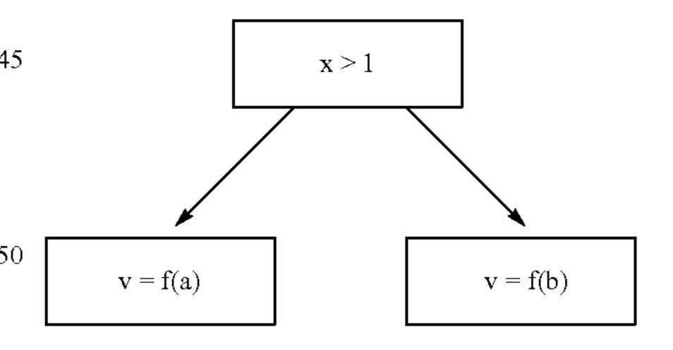
Thus, for each source code statement, code parser 208 uses the instruction logic to determine the number of nodes that CFG generator 210 generates and the connections between each node. CFG generator 210 then connects the individual CFGs that represent a control flow of each statement into a CFG that represents the control flow of browser extension 112.
