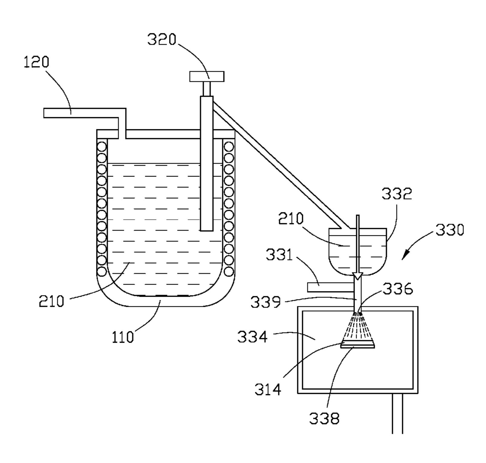
Providing a molten magnesium-based material
