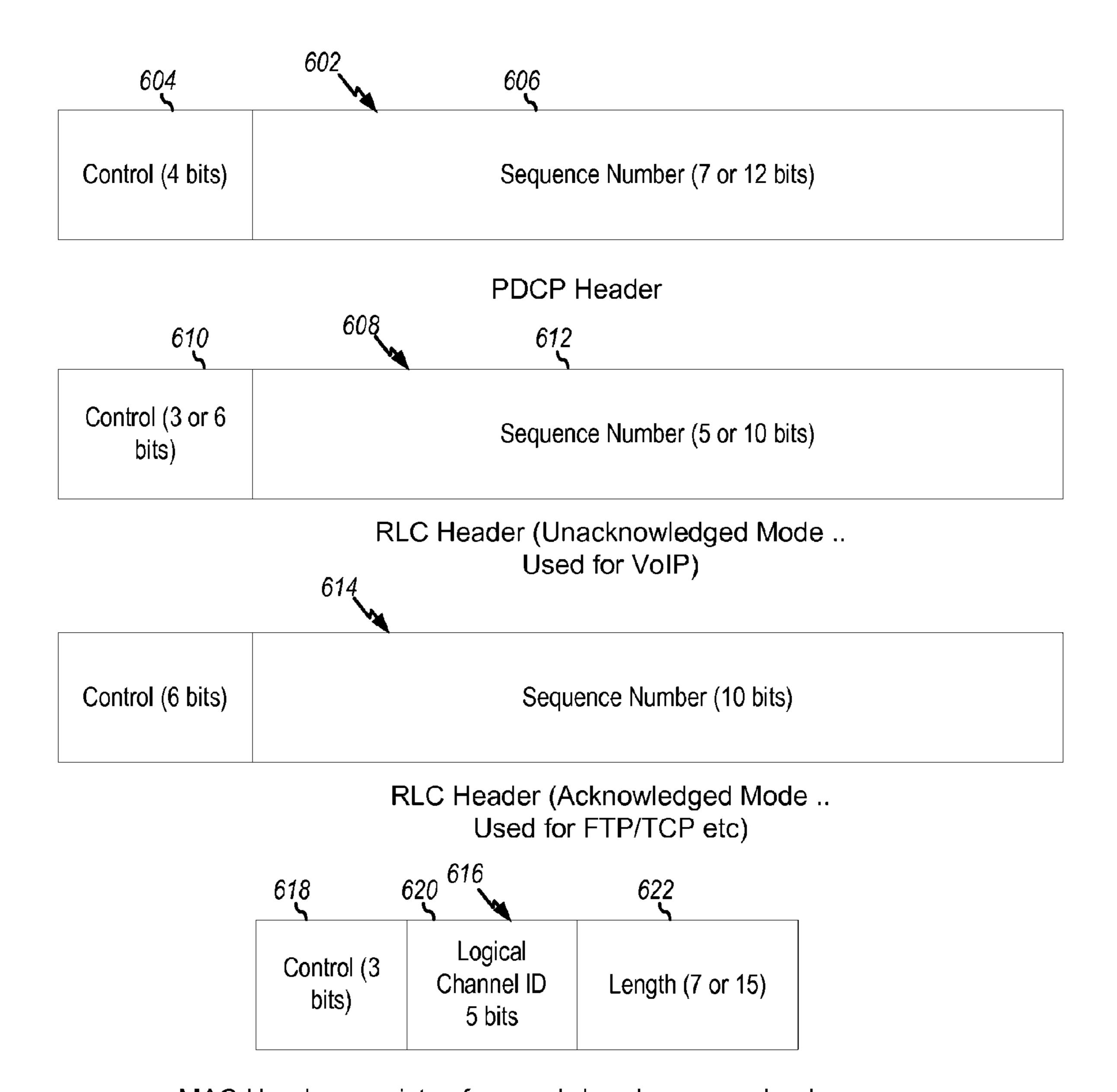
MAC Header consists of one sub-header per payload
