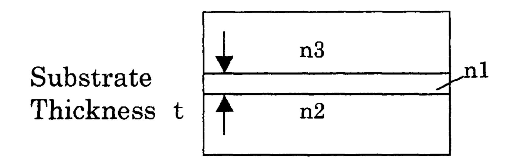
Calculating condition: n2, n3 are sufficiently thick
