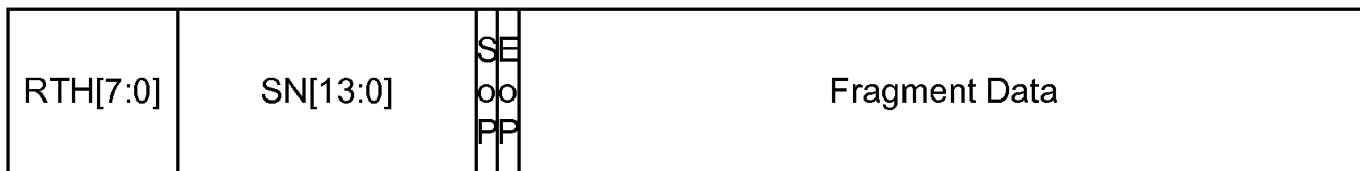
Standardized PAF Fragment with additional Retransmission Header RTH
