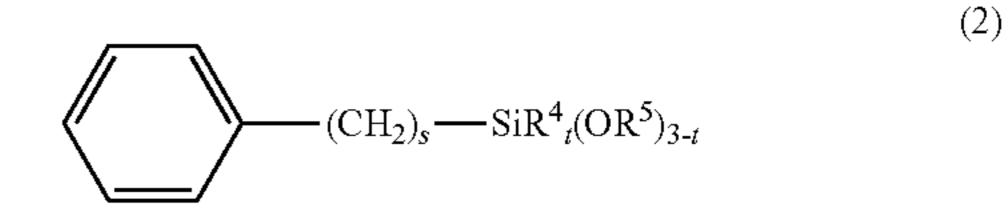
(in the formula (2), R<sup>4</sup> is an alkyl group having 1 to 3 carbon atoms or a phenyl group which may have a substituent; R<sup>5</sup> is a hydrogen atom or a hydrocarbon group having 1 to 10 carbon atoms; s is an integer of 0 to 6; and t is an integer of 0 to 2.
