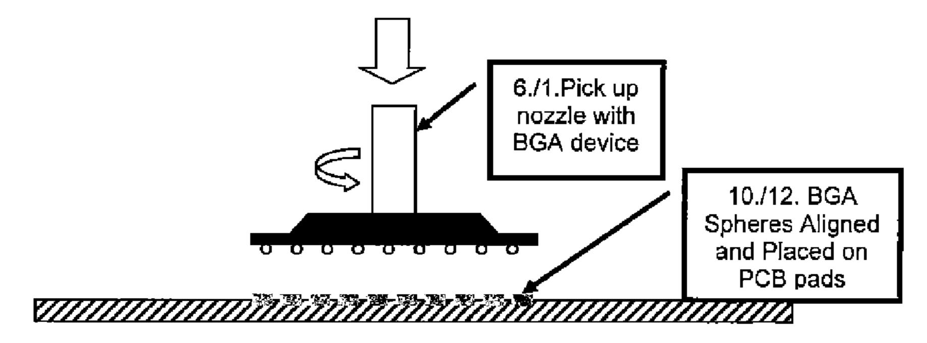
Step 3: Fluxed BGA is moved into correct alignment with PCB pads and placed on pads using vacuum nozzle placement head, with rotational alignment of component or board if required
