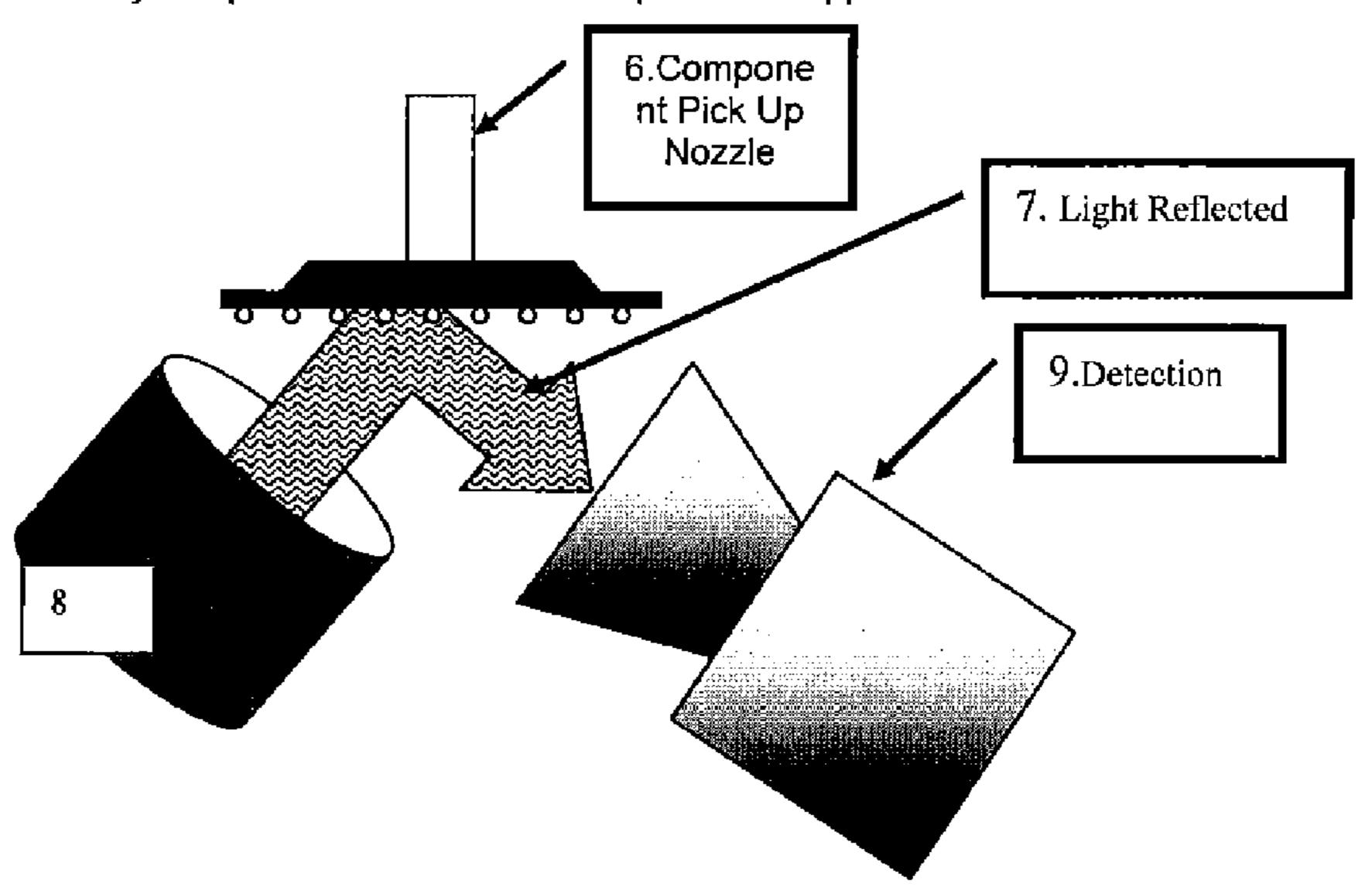
Step 2: BGA is moved into position over light source and detection camera to ensure flux is present on BGA spheres
