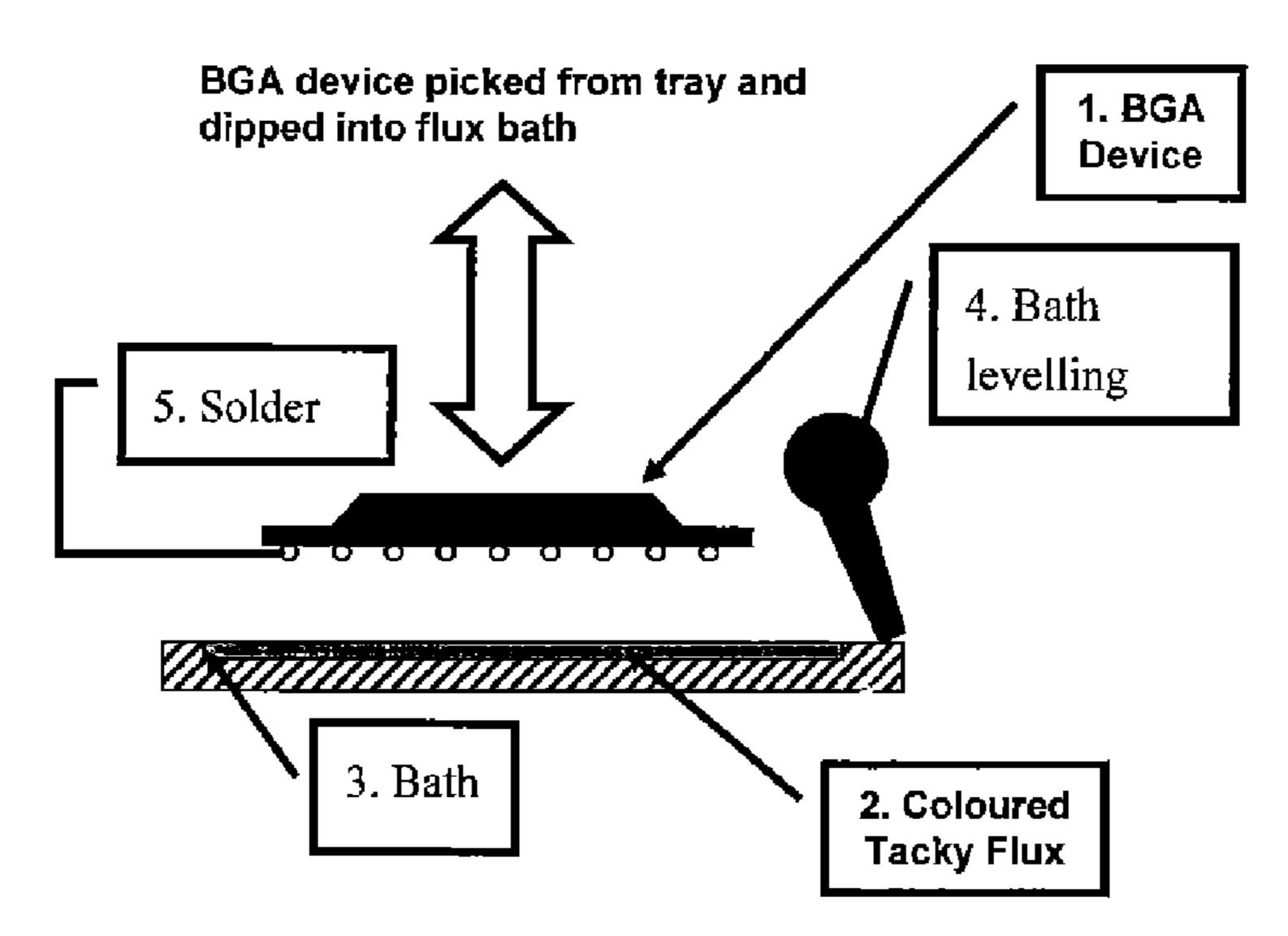
Step 1: BGA is picked from storage tray by vacuum cup (not shown) and dipped in flux bath. Bath is levelled by scraper blade after each component is dipped
