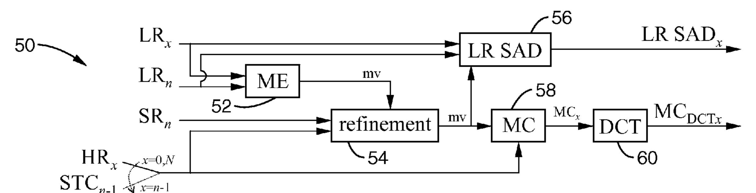
LR<sub>x</sub> is low-resolution video picture, x=0, n-1, or N HR<sub>x</sub> is high-resolution still for x=0 or N SR<sub>n</sub> is the super-resolved video picture STC<sub>n-1</sub> is the previous STC output
