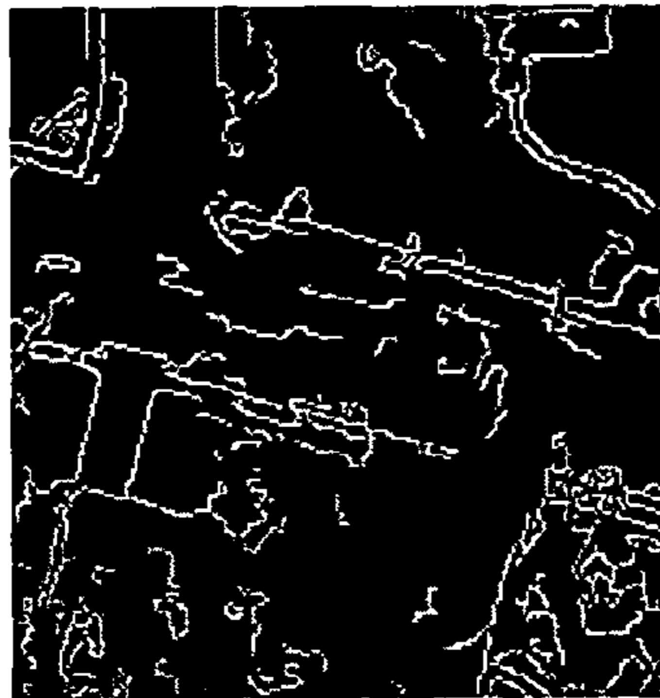
Detected edges by Canny edge detector
