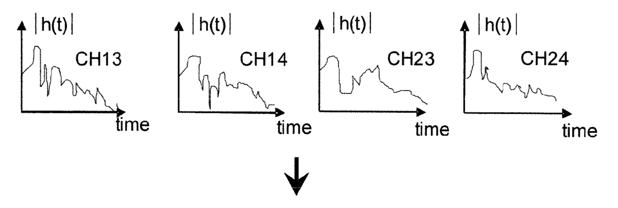
Power delay profile averaged over time and antennas
