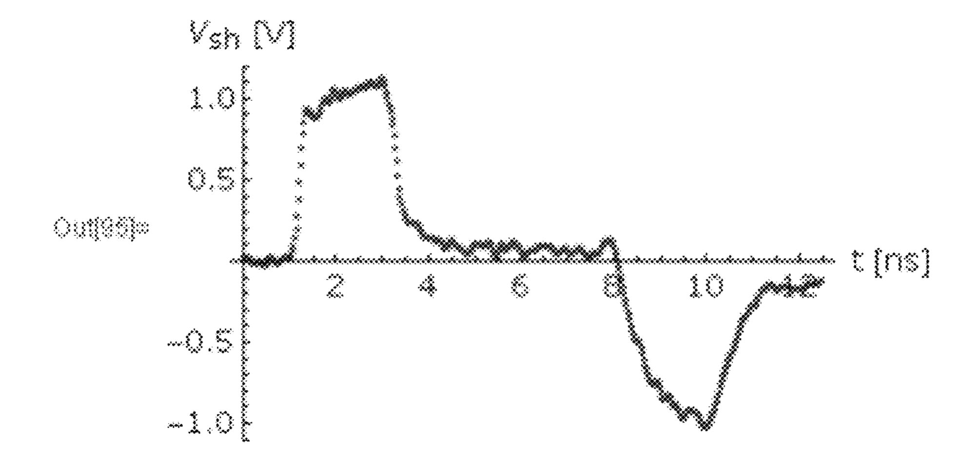
$R_s$  &  $L_s$  parasitic extraction from VF TLP waveforms, Intercept- $R_s$ , Slope- $L_s$
