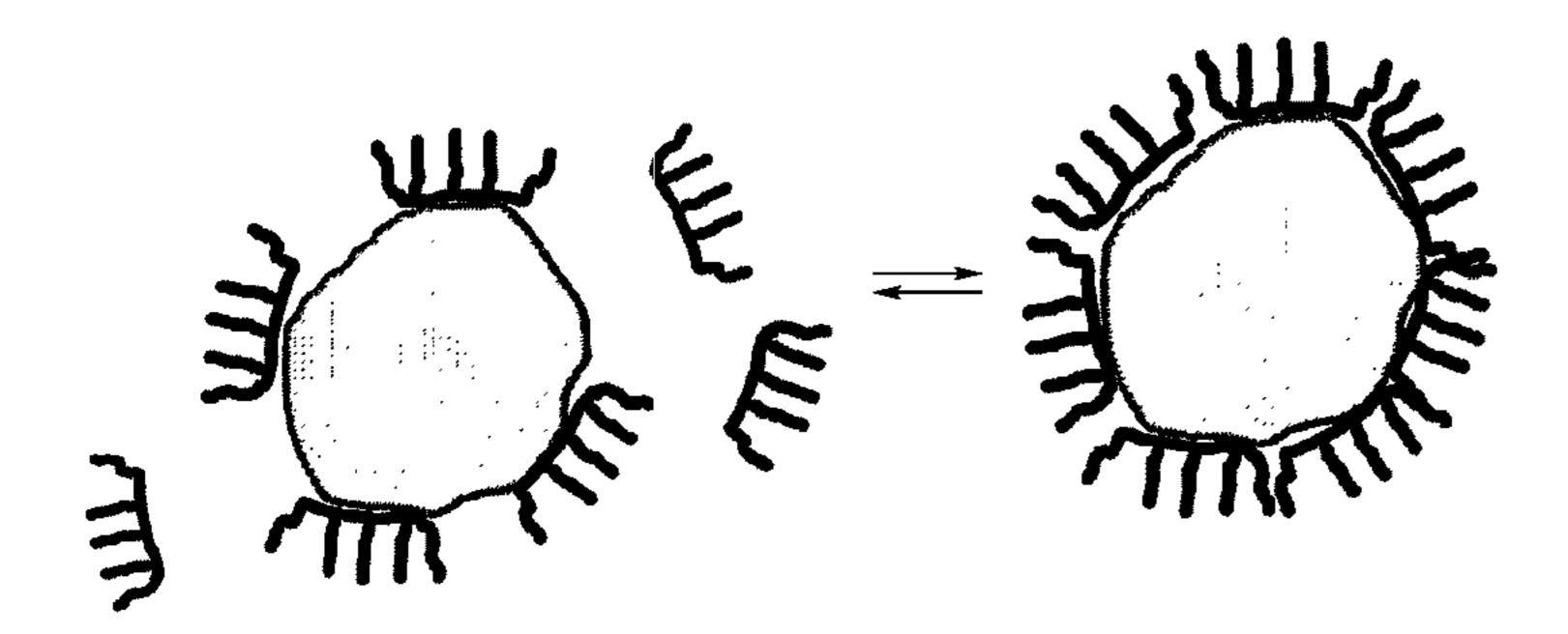
If the dispersant can be crosslinked or chain extended to a higher molecular weight after adsorption to the pigment surface, it will then be locked in place or become less soluble in the continuous phase and therefore much less able to desorb. Therefore, the stability of the pigment dispersion is much less 20 prone to be adversely affected by the changes in environment (vehicle composition, temperature, etc.) as discussed above.
