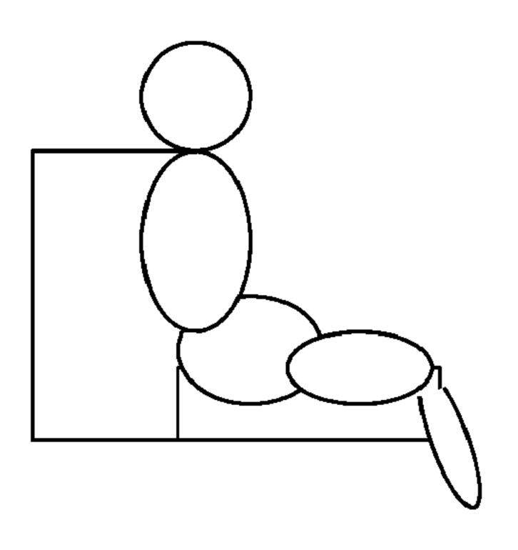
The subject is lowered into the L-shaped foam and an impression is taken which can vary with the height and posture of the subject. The foam could extend to capture the cervical and cranial imprint. A correspondingly tall wheelchair would be needed to received the mold.
