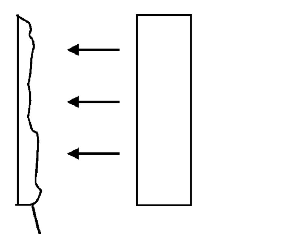
The foam is pressed against the face of the unfinished seating apparatus of the plane or automobile, making a mirror image which can then be over-sprayed in the same manner as mold taken from the human body
