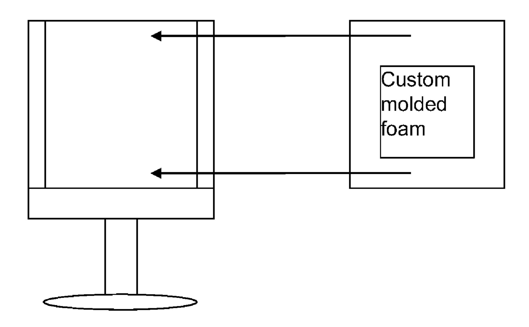
Using foam to create impression of aircraft or automobile seat
