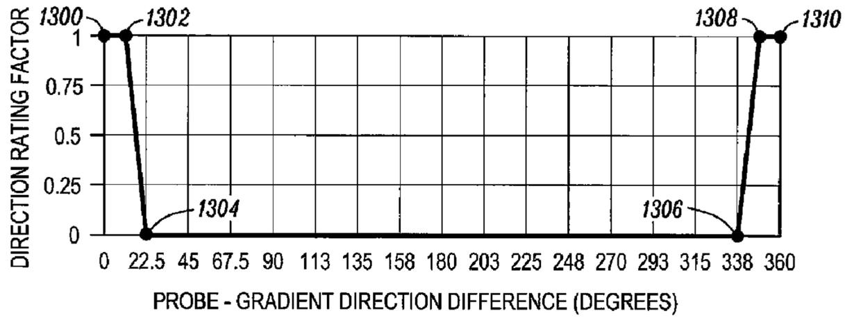
DIRECTION RATING FACTOR FUNCTION, CONSIDER POLARITY CASE
