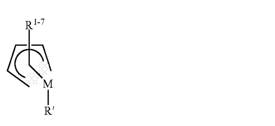
In this embodiment, y equals 0. That is, the organometallic compound comprises only an open pentadienyl ligand and the R' ligand. Furthermore, in at least one embodiment, at least 5 of R<sup>1-7</sup> are hydrogen groups. In other words, besides the MR' functional group, the Op group has two substituents. The two substituents preferably are a methyl or ethyl group. In at least one embodiment, the precursor has the formula shown in (3) where R' is bis((trimethylsilyl)acetylene.
