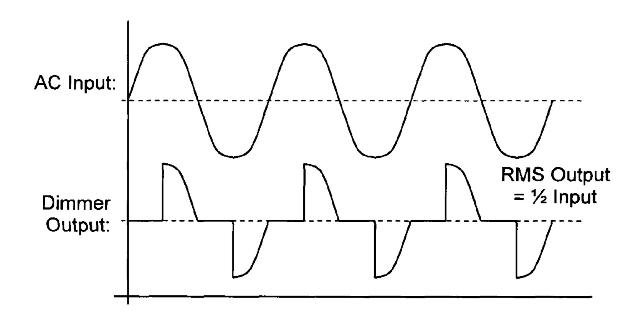
Fig. 6 Reverse Phase Control AC Waveform With Dimmer Set To Half
