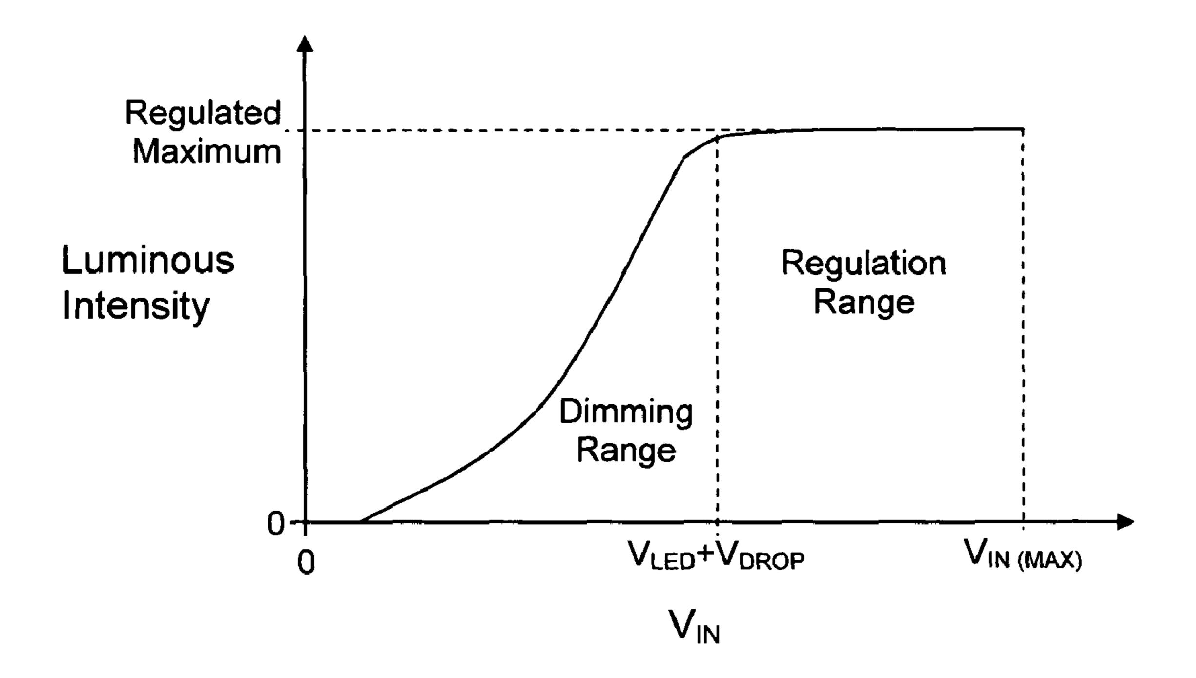
Fig. 4 Non-Linear Dimming Response In A Linear Regulated LED
