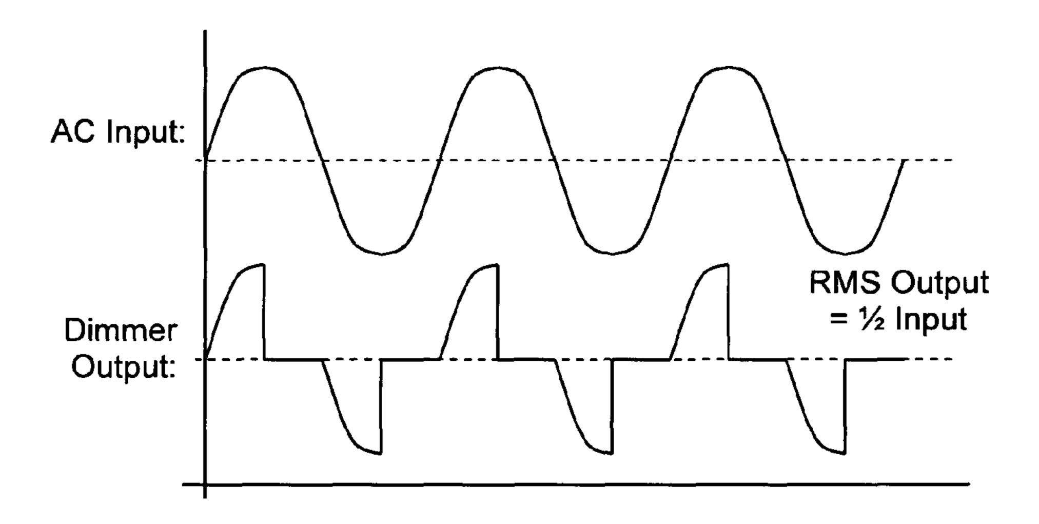
Fig. 7 AC Waveform From Autotransformer Set To Half
