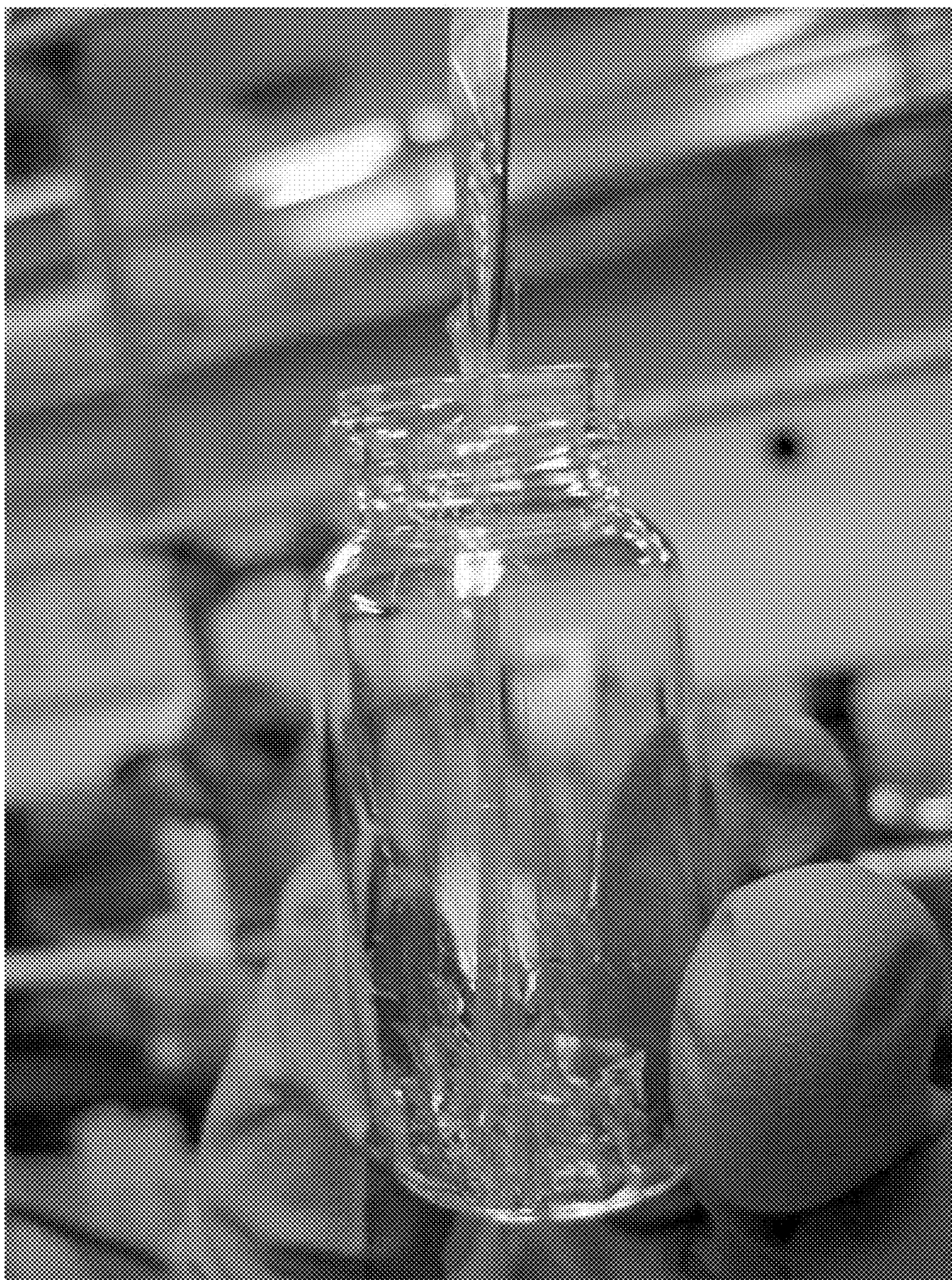
Figure 1. Qualitative test for high molecular weight polyurethane.
