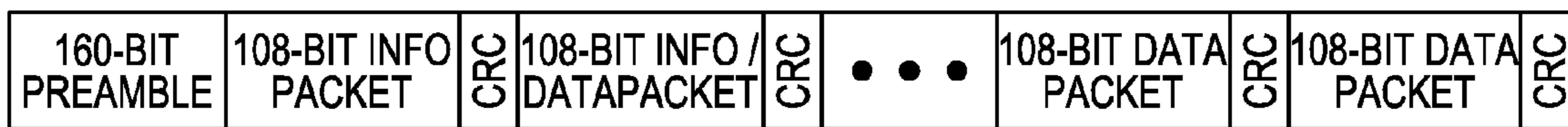
STRUCTURE OF UPLINK BURST
