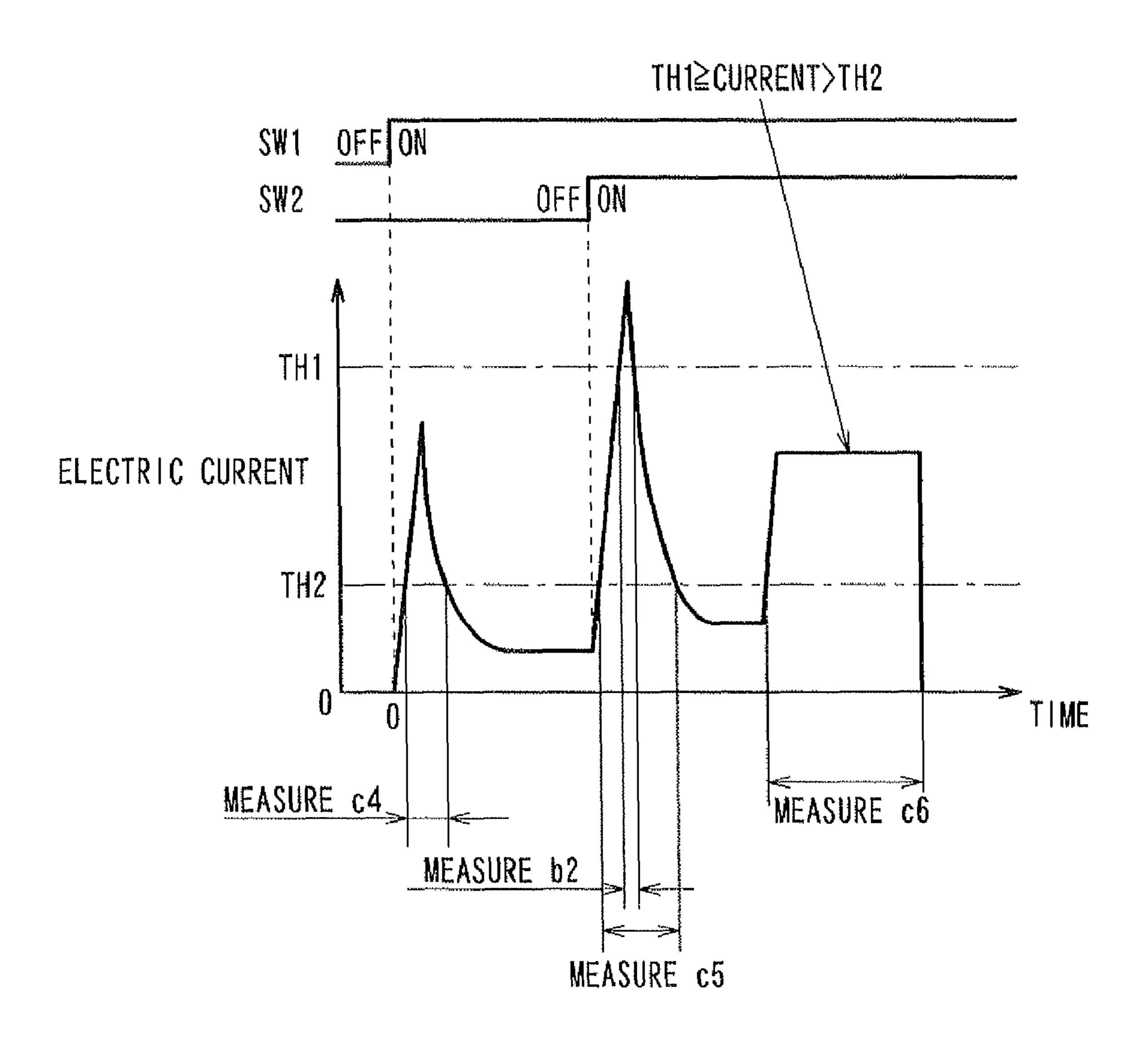
b2<T1 → NO DETECT c4, c5<T2 → NO DETECT c6≥T2 → OVERCURRENT DETECT
