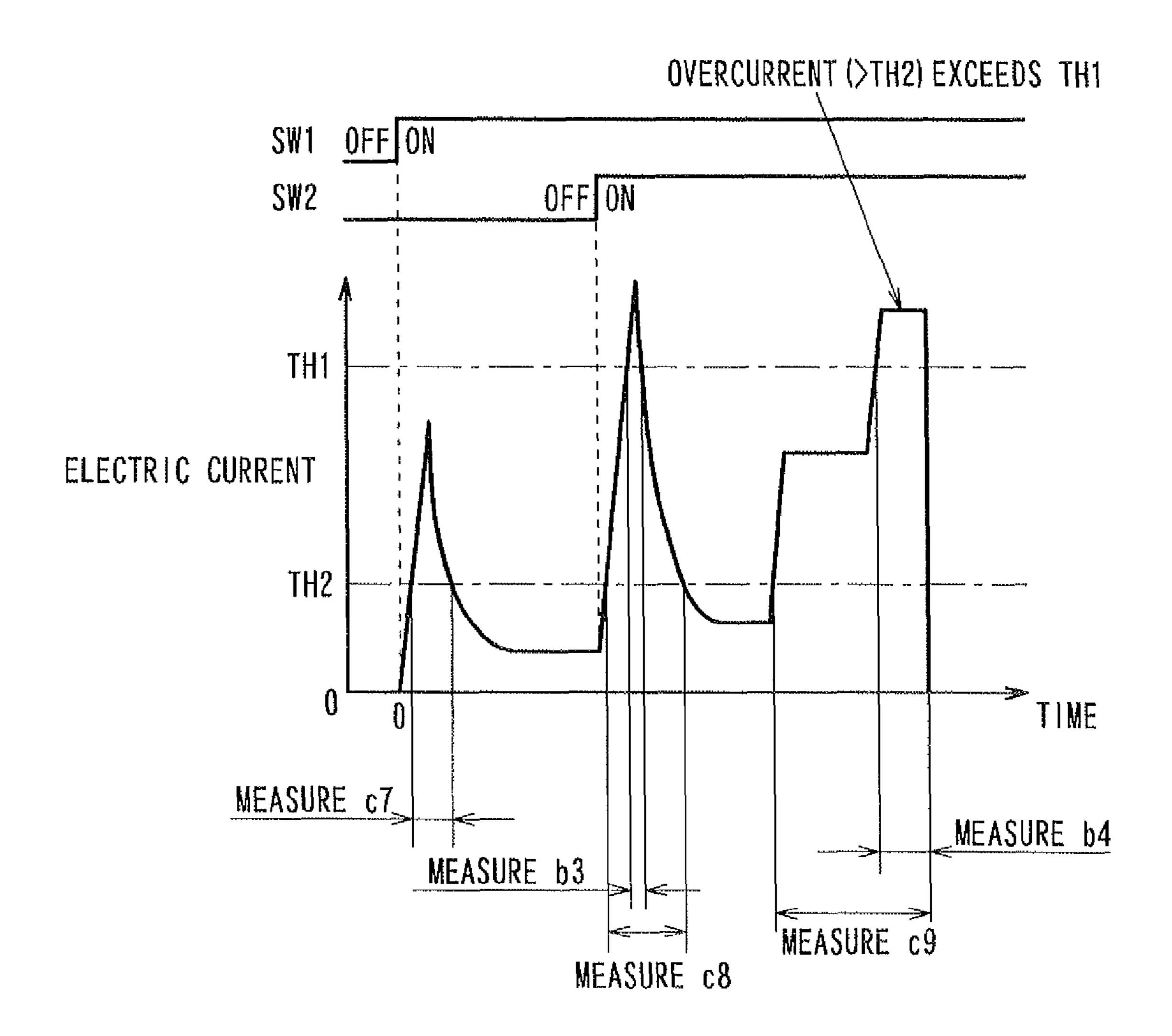
b3<T1 → NO DETECT c7, c8<T2 → NO DETECT b3<T1 → NO DETECT c9≥T2 → OVERCURRENT DETECT
