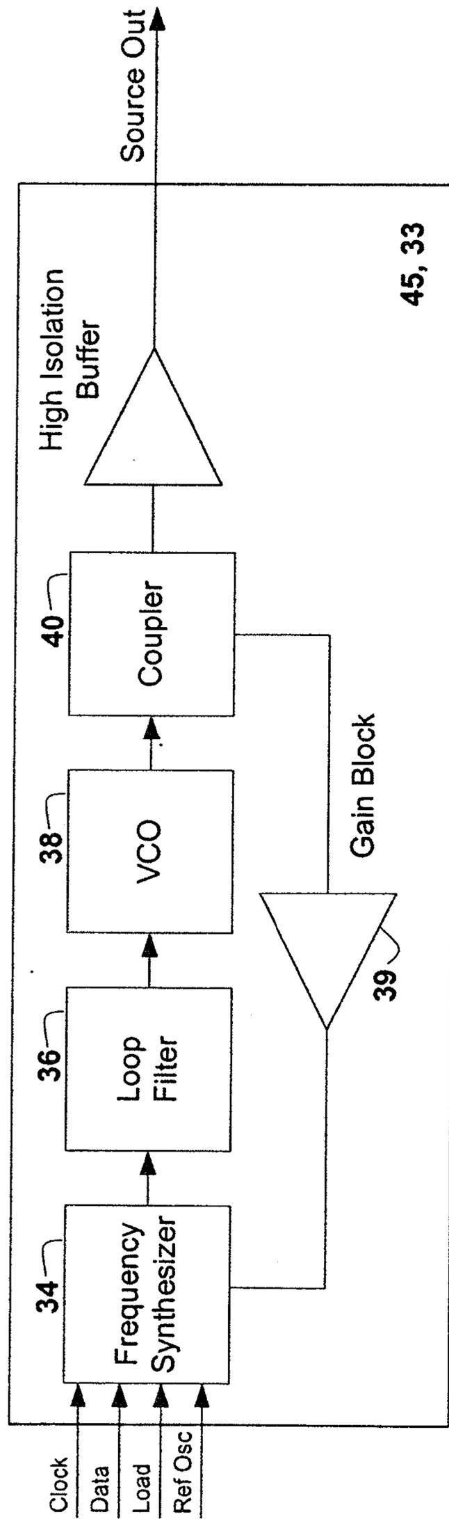
Figure 5 Synthesized Source Block Diagram
