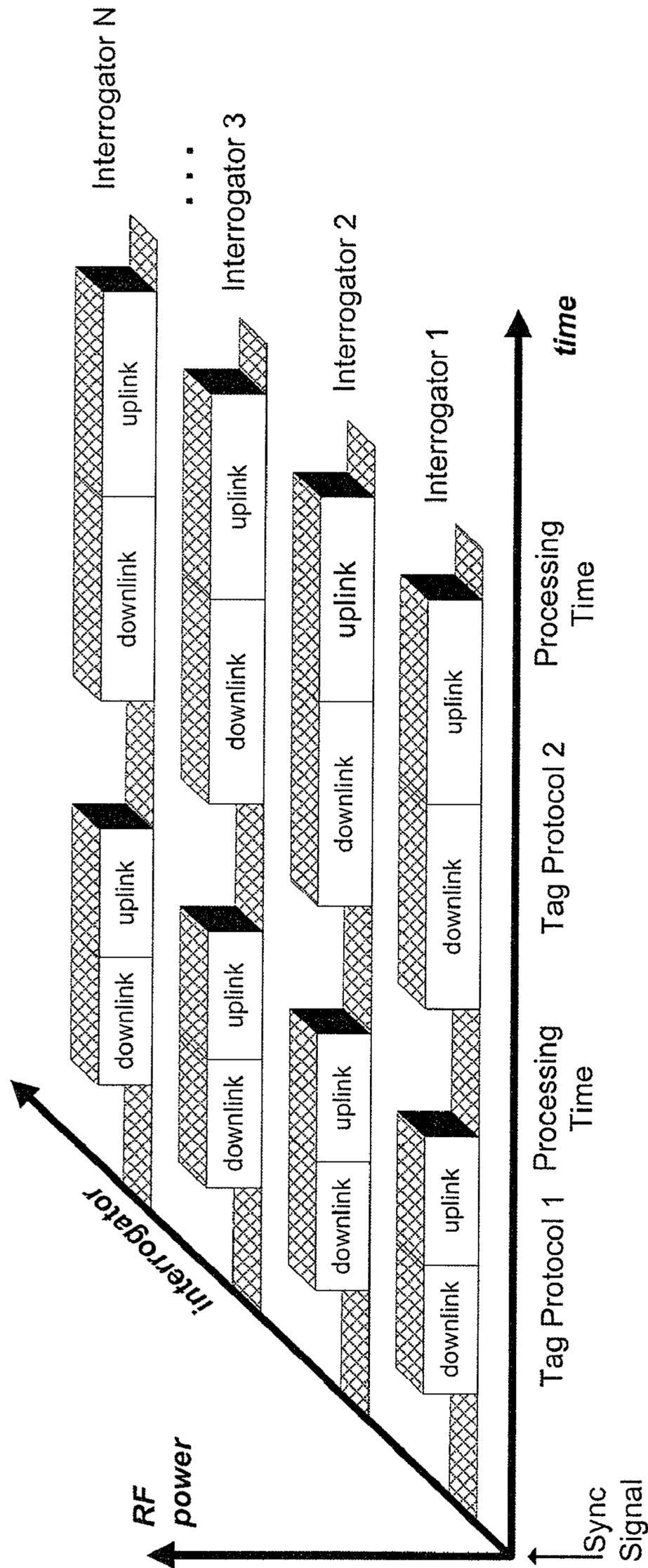
Figure 3(a) – Step Lock Timing Diagram
