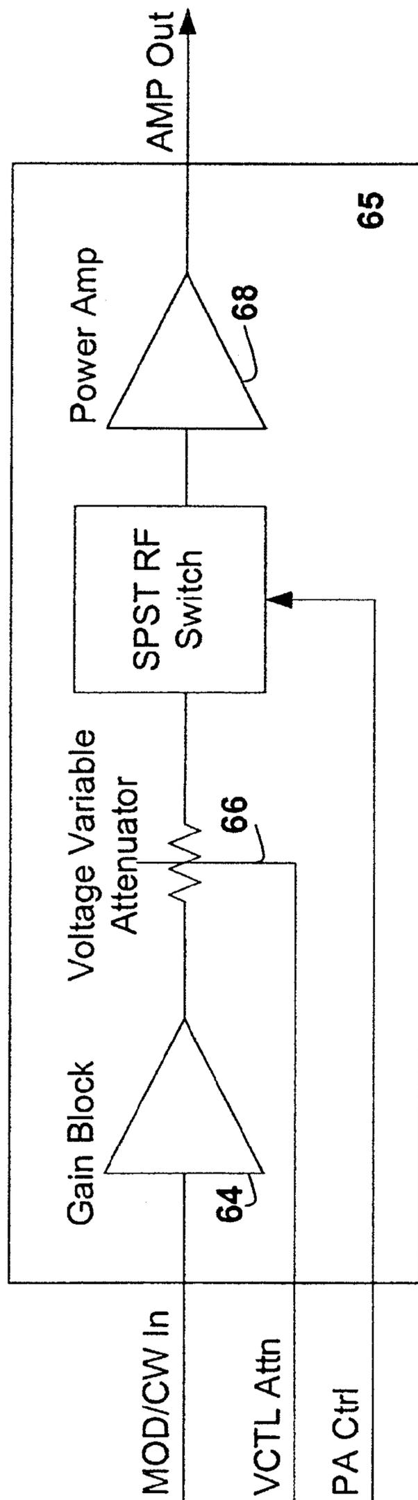
Figure 8 Power Amplifier Block Diagram
