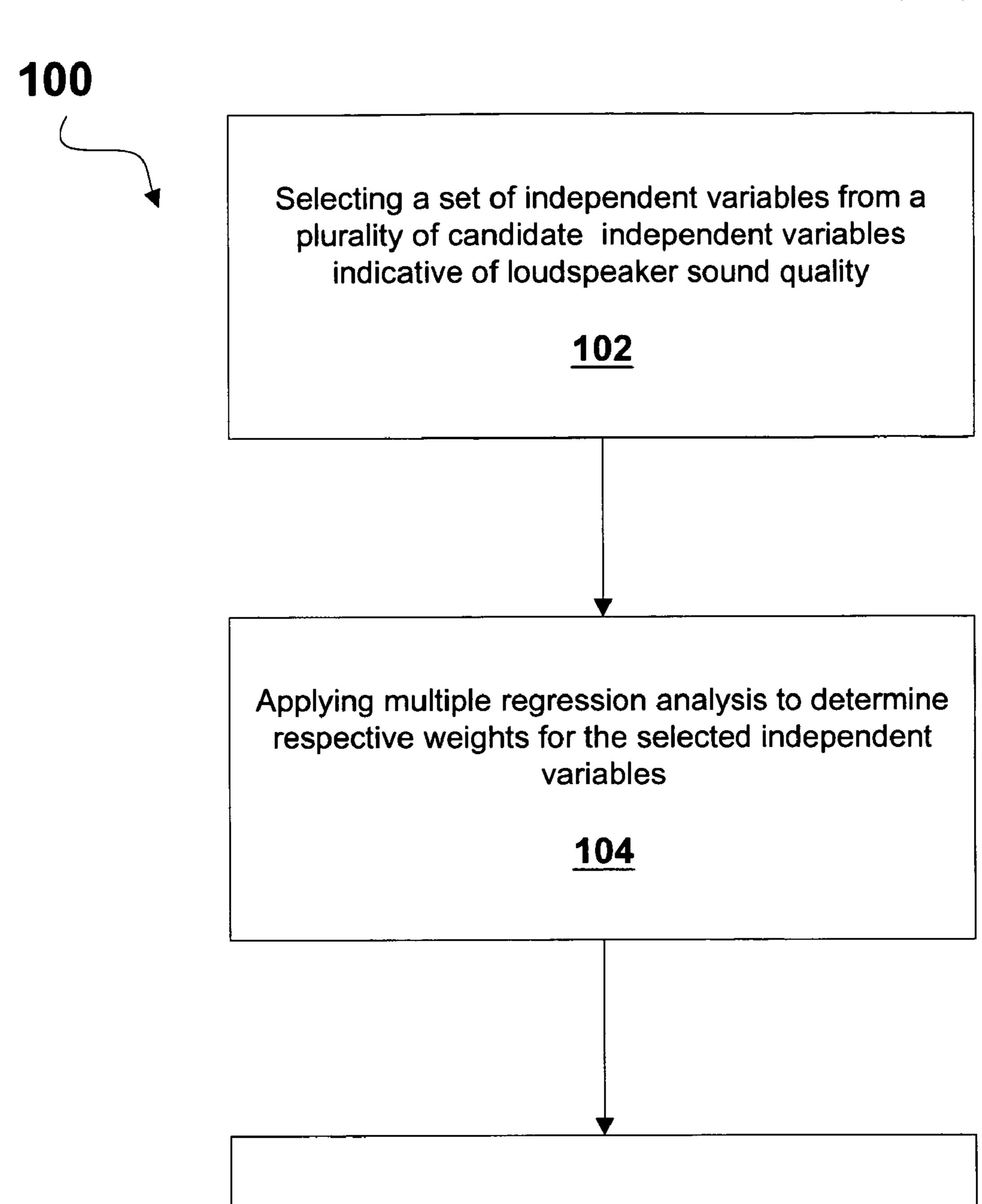
Arranging the weighted independent variables into a linear equation into a linear equation representative of the predicted loudspeaker preference rating
