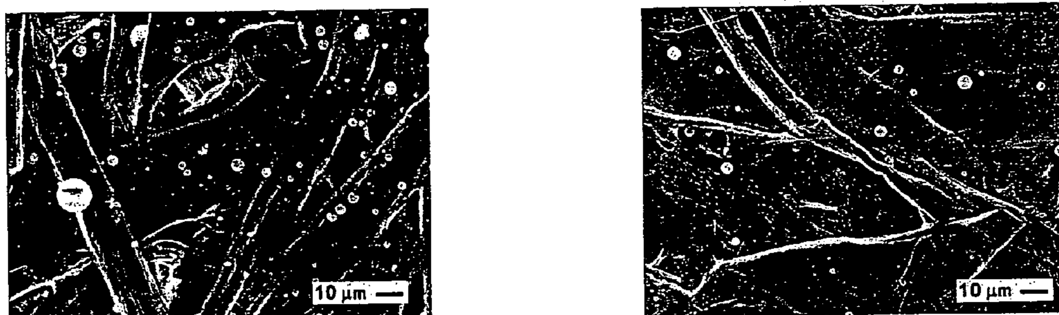
Figure 5: A SEM of P2 with a magnification of 750x, left: with coating weight 0,1 g/m 2 , right: with coating weight 0,01 g/m 2
