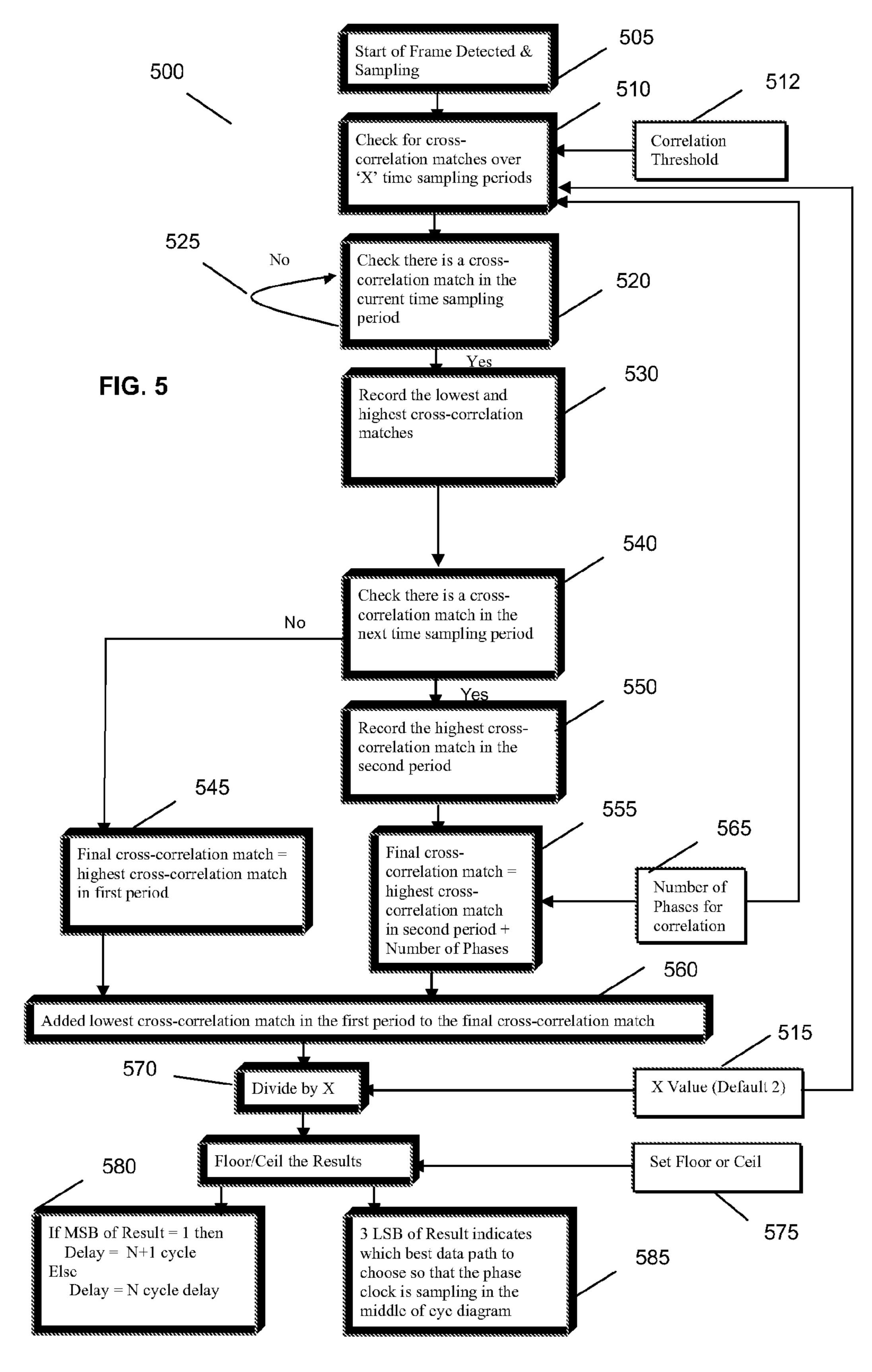
Delay – How many bit periods it took to make the decision on the correct clock phase and data path selection. It determines how far along the data pipe the incoming data has preceded.
