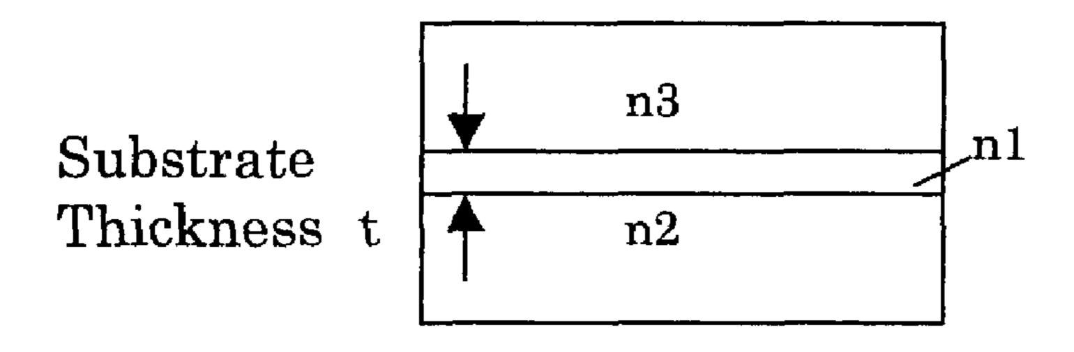
Calculating condition: n2, n3 are sufficiently thick
