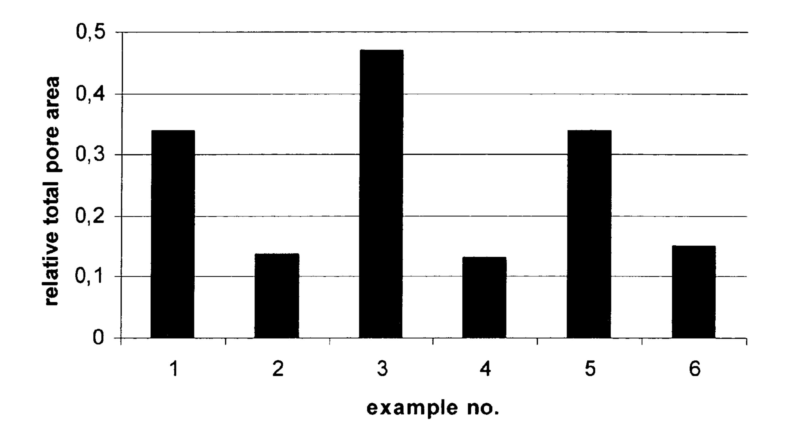
Results from Nitric-Acid Vapour corrosion resistant tests according to ASTM B735-95.
