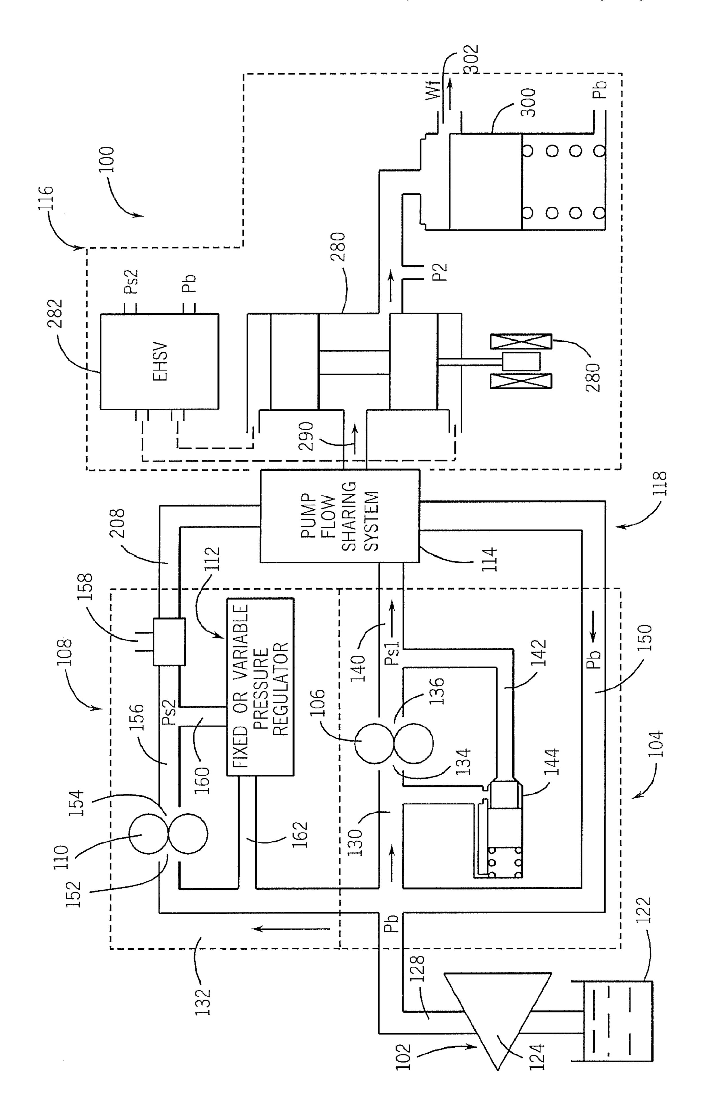
FUEL DELIVERY AND CONTROL SYSTEM INCLUDING A POSITIVE DISPLACEMENT ACTUATION PUMP WITH A VARIABLE PRESSURE REGULATOR SUPPLEMENTING A FIXED DISPLACEMENT MAIN FUEL PUMP
