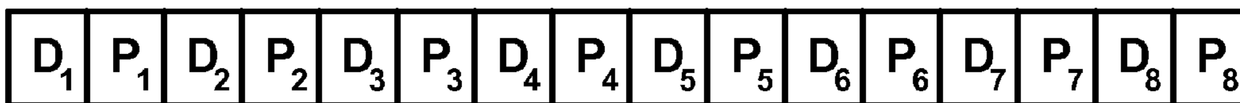
Fig. 4 BIT ORDER IN 1/2 RATE M/H FOR SCCC
