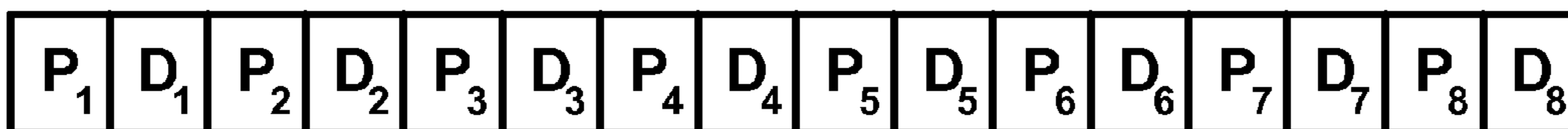
Fig. 5 BIT ORDER IN 1/2 RATE M/H FOR PCCC
