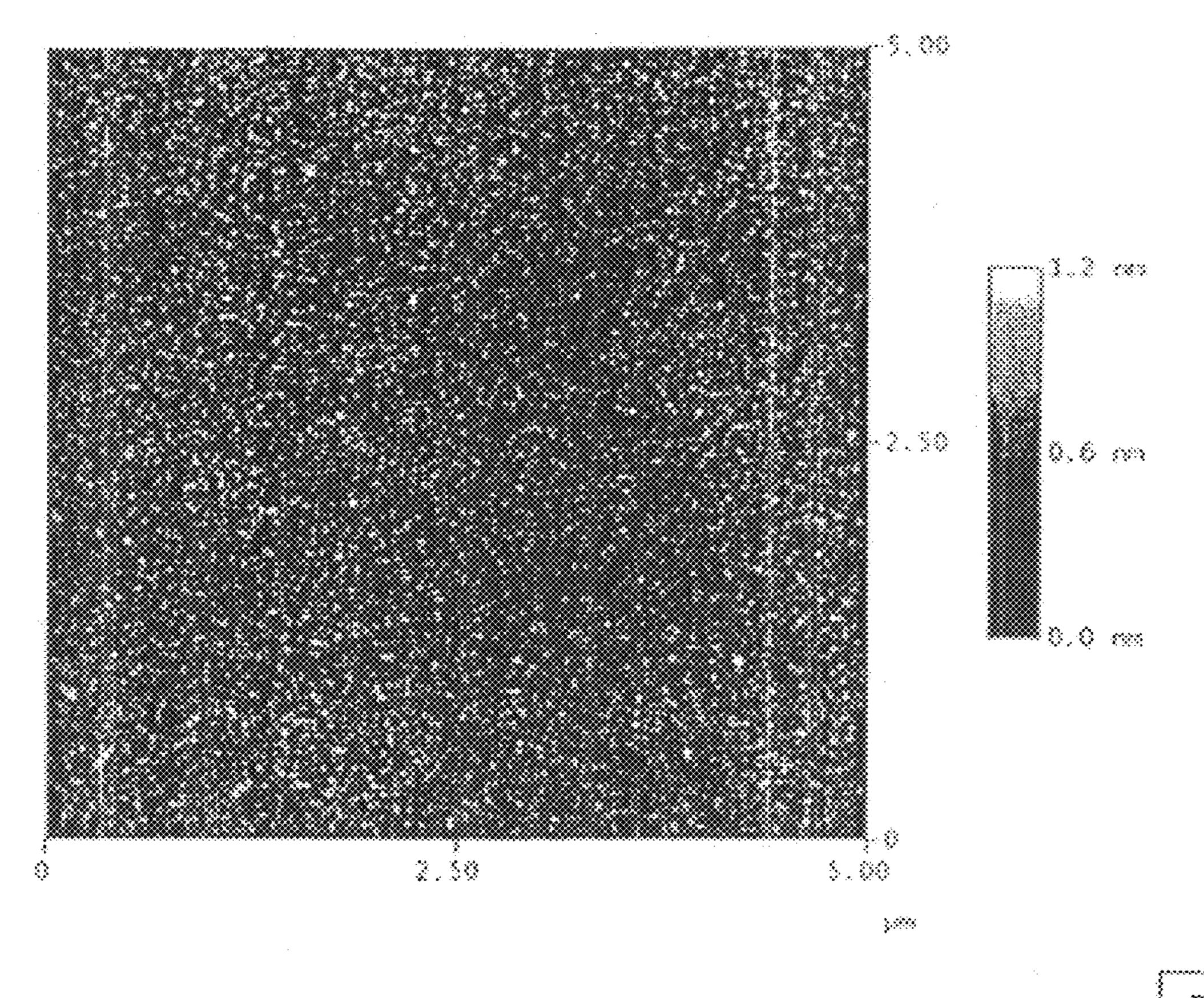
Roughness analysis: Mean roughness = 0.059 nm Max. Height = 2.60 nm
