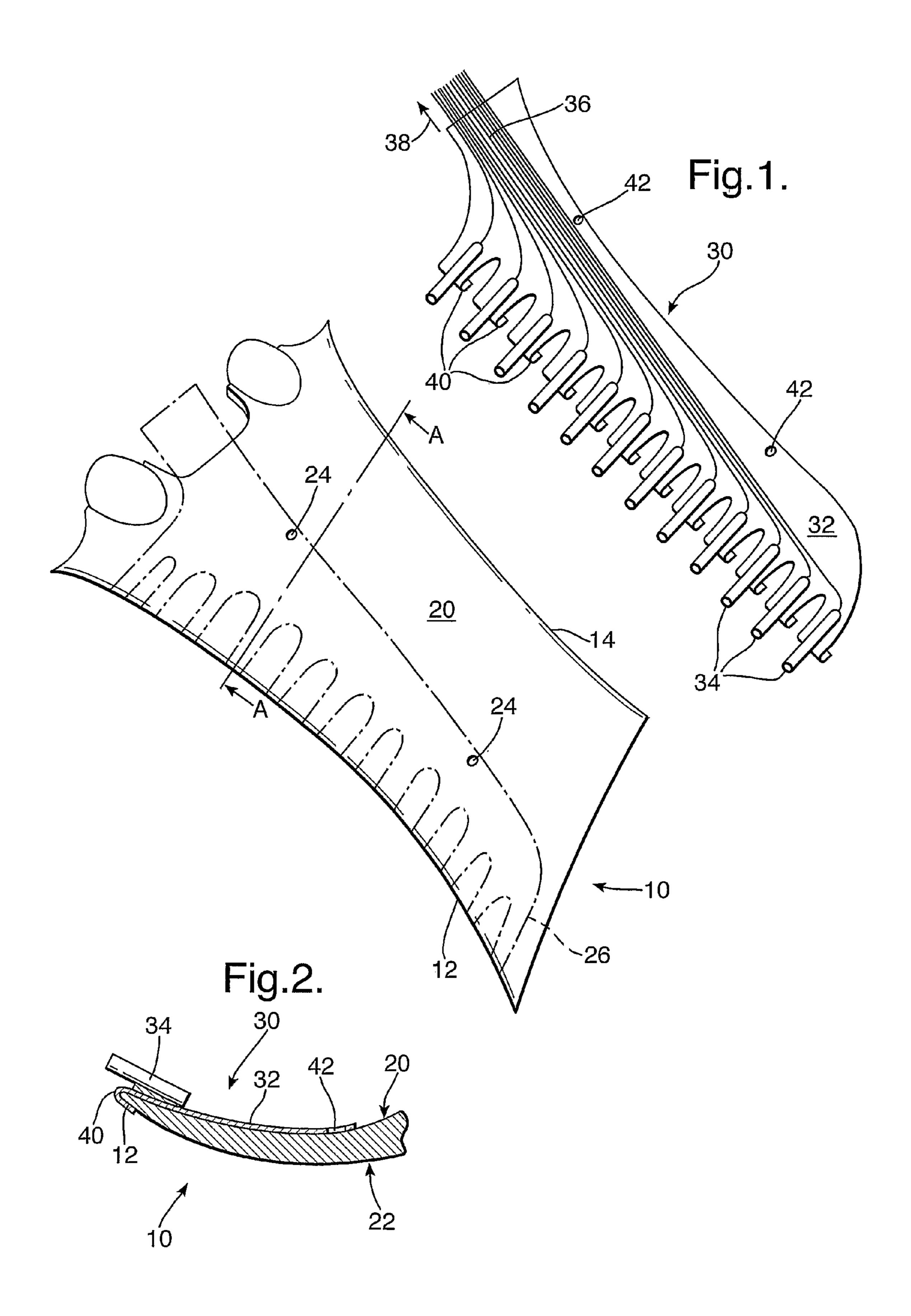
This invention relates to instrumentation, and particularly to measurement devices intended for use on stationary components of gas turbine engines.
