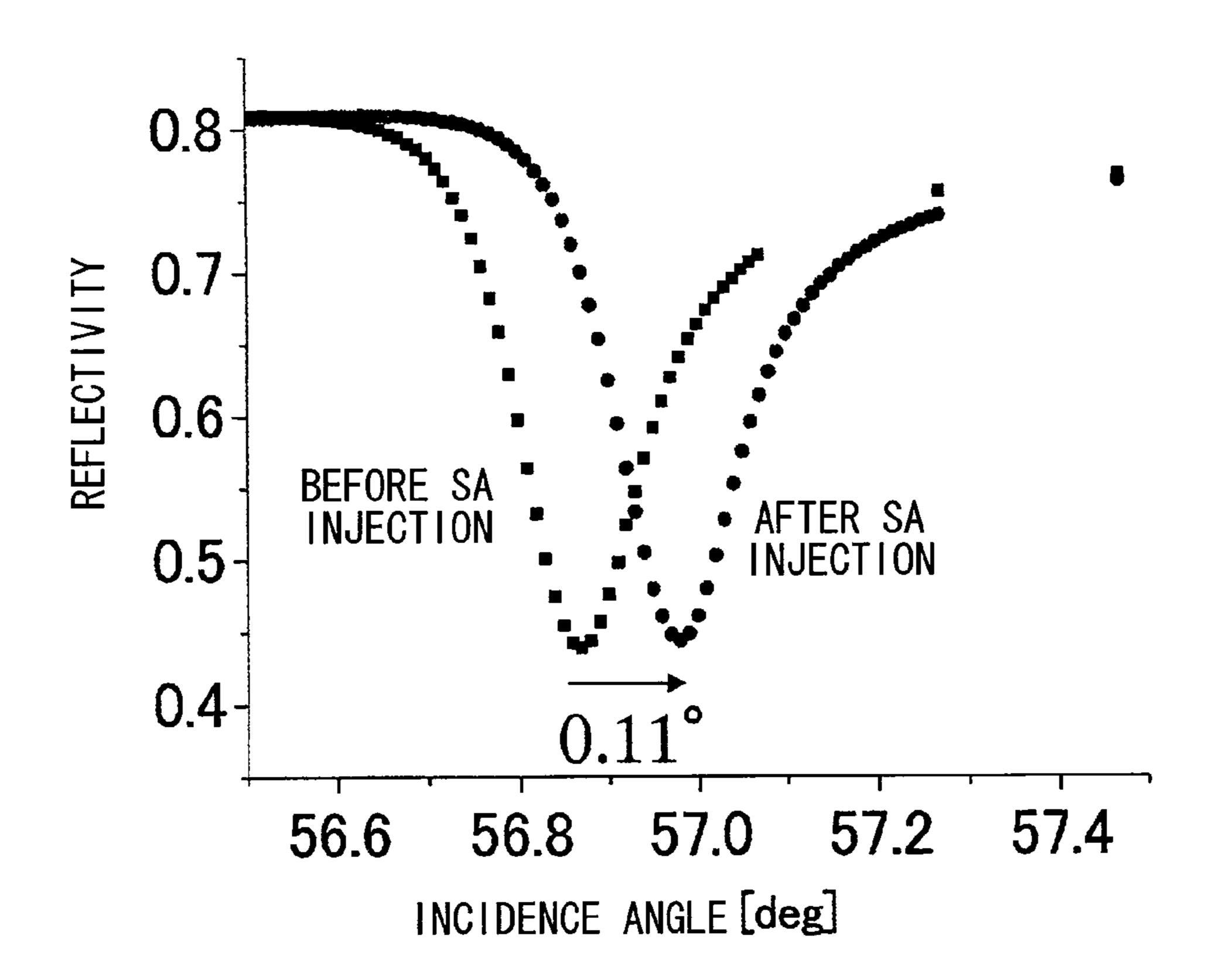
CHANGE IN INCIDENCE ANGLE DEPENDENCY OF INTENSITY OF REFLECTED LIGHT CAUSED BY SPECIFIC ADSORPTION OF STREPTOAVIDIN MEASURED BY USING SPECIMEN B
