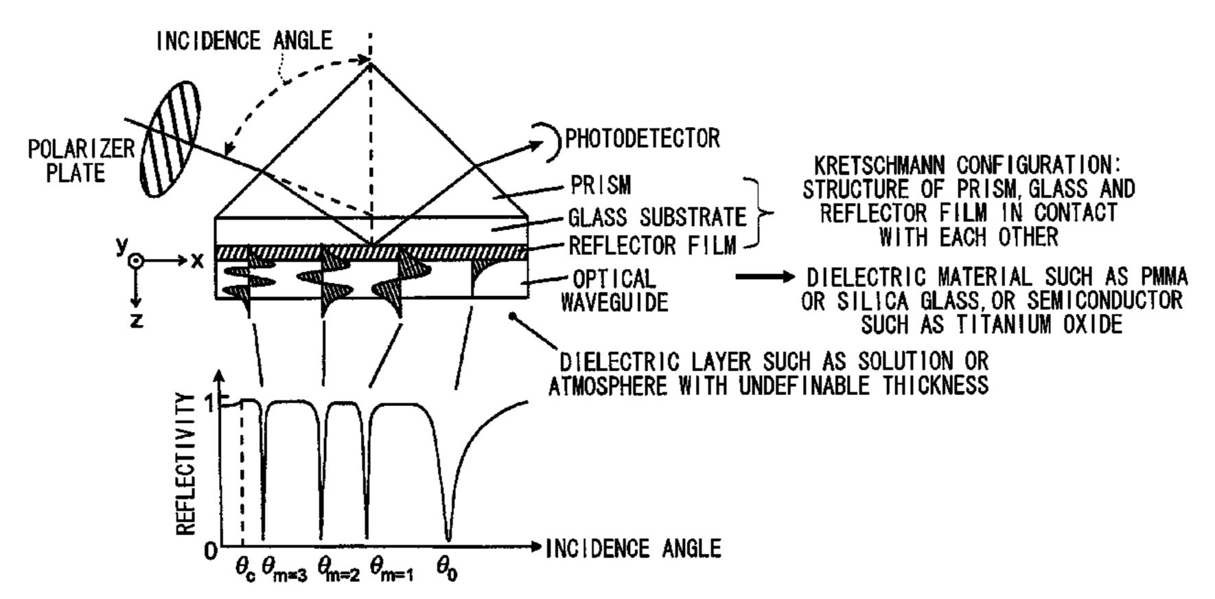
$\theta_{m=1}$  angles at which the incident light that illuminates the reflector film couples with the optical waveguide modes and propagates in the optical waveguide (EVANESCENT WAVE)
