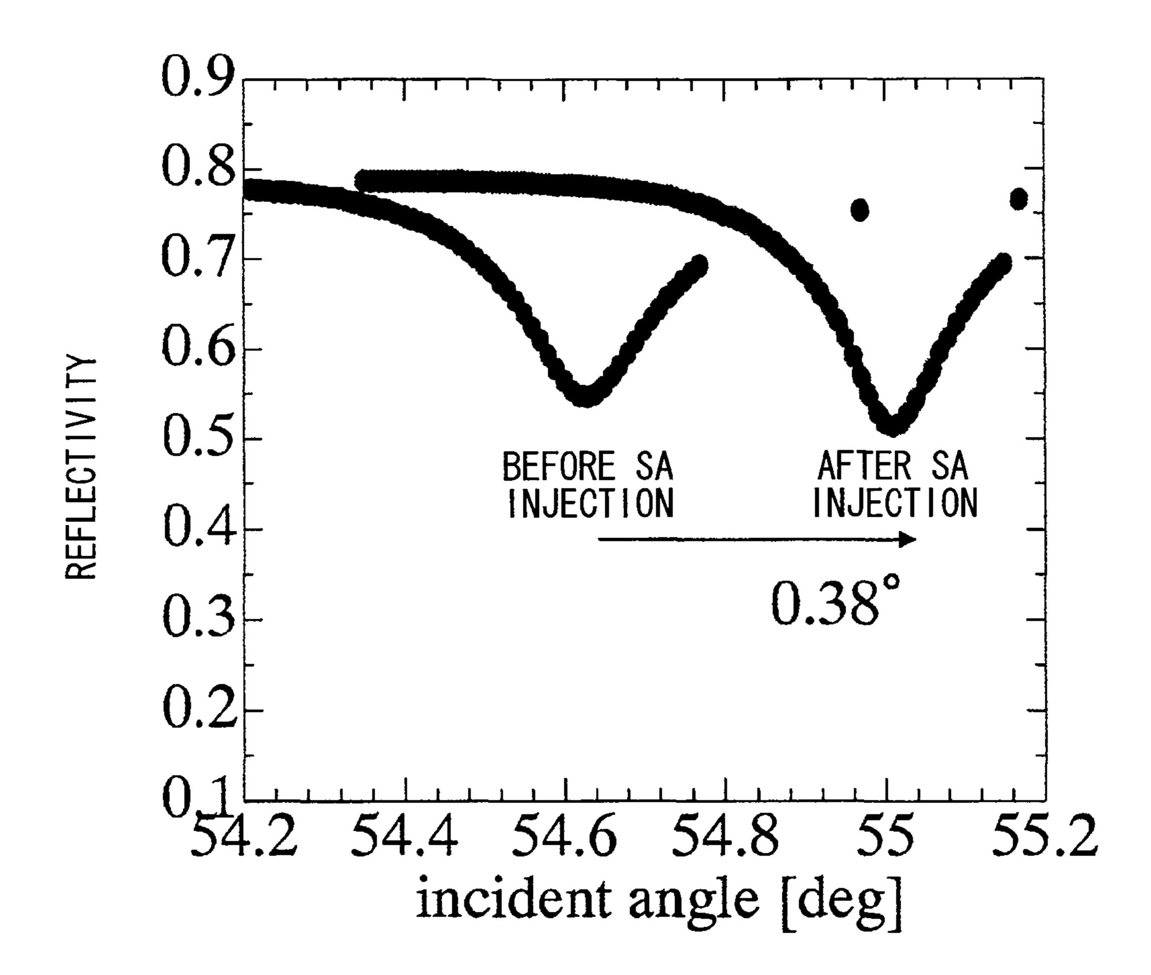
CHANGE IN INCIDENCE ANGLE DEPENDENCY OF INTENSITY OF REFLECTED LIGHT CAUSED BY SPECIFIC ADSORPTION OF STREPTOAVIDIN MEASURED BY USING SPECIMEN D
