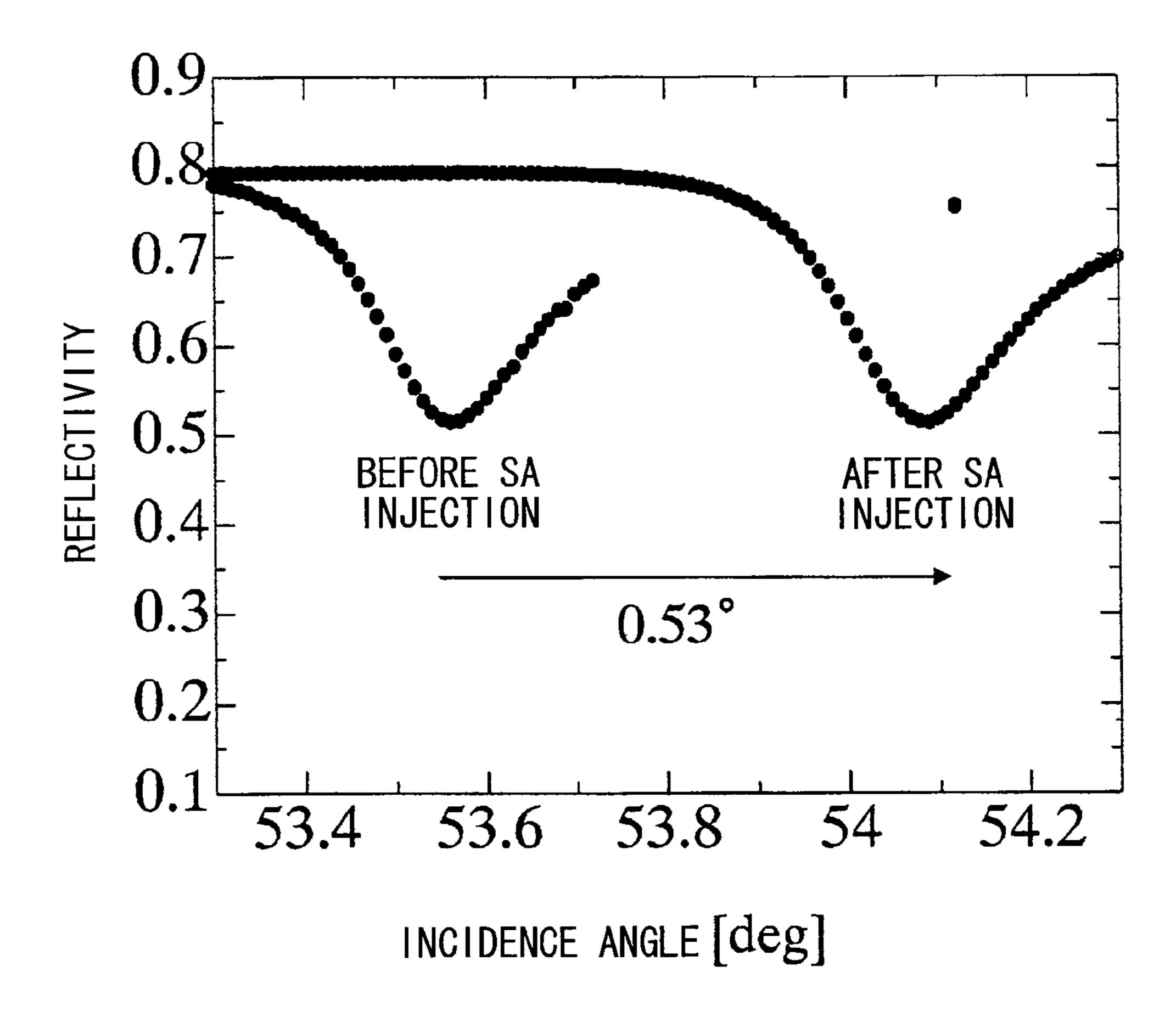
CHANGE IN INCIDENCE ANGLE DEPENDENCY OF INTENSITY OF REFLECTED LIGHT CAUSED BY SPECIFIC ADSORPTION OF STREPTOAVIDIN MEASURED BY USING SPECIMEN E
