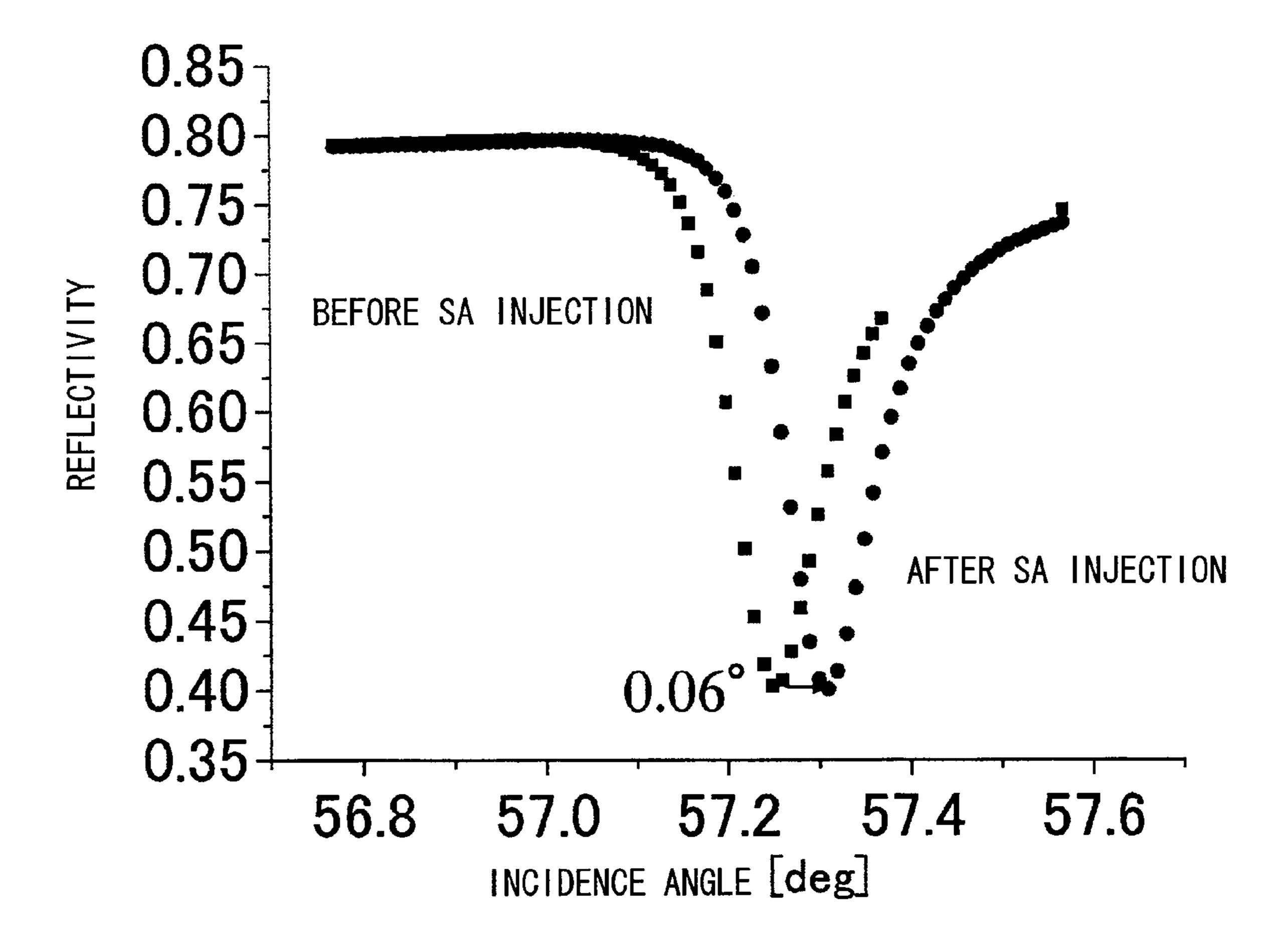
CHANGE IN INCIDENCE ANGLE DEPENDENCY OF INTENSITY OF REFLECTED LIGHT CAUSED BY SPECIFIC ADSORPTION OF STREPTOAVIDIN MEASURED BY USING SPECIMEN A
