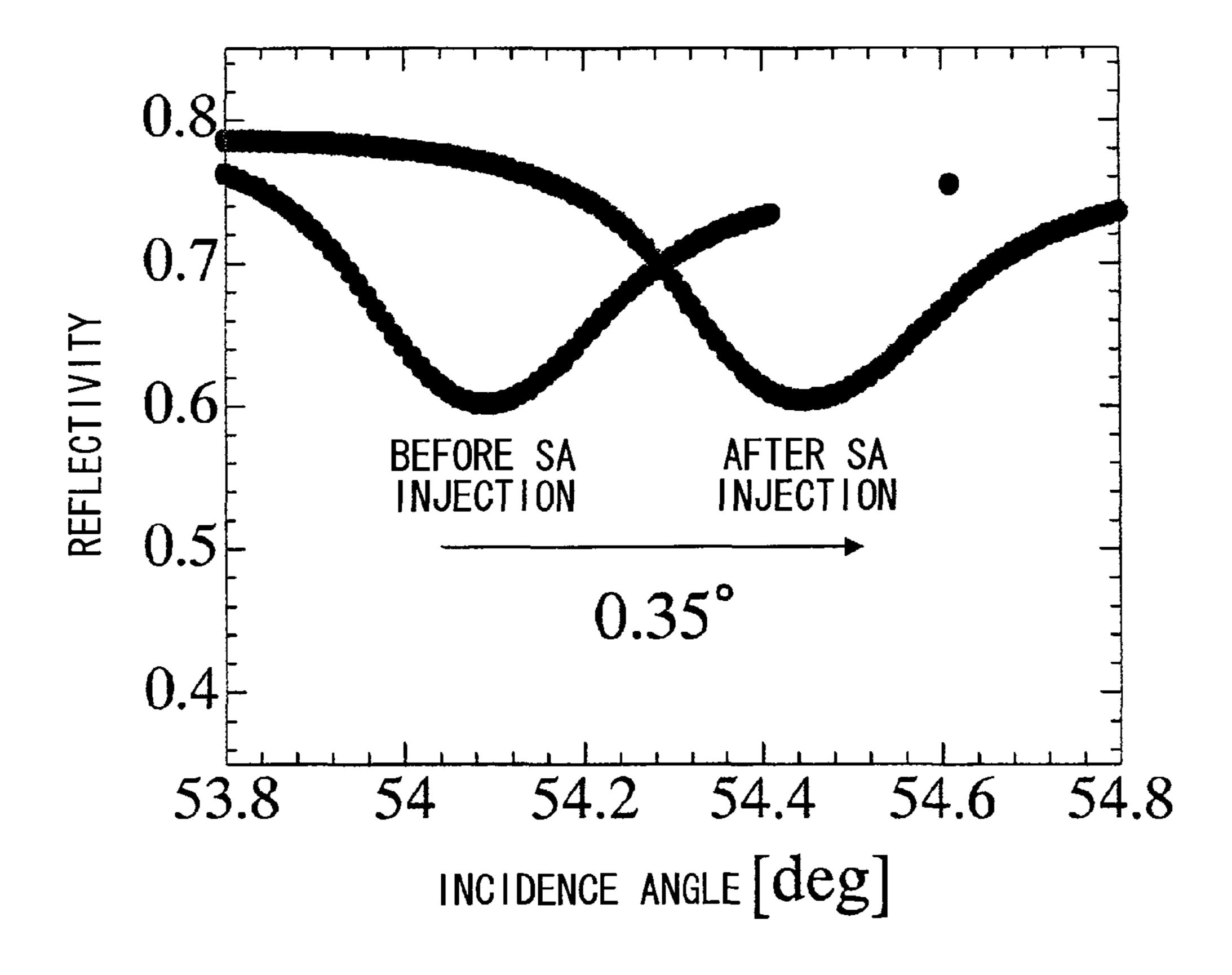
CHANGE IN INCIDENCE ANGLE DEPENDENCY OF INTENSITY OF REFLECTED LIGHT CAUSED BY SPECIFIC ADSORPTION OF STREPTOAVIDIN MEASURED BY USING SPECIMEN C
