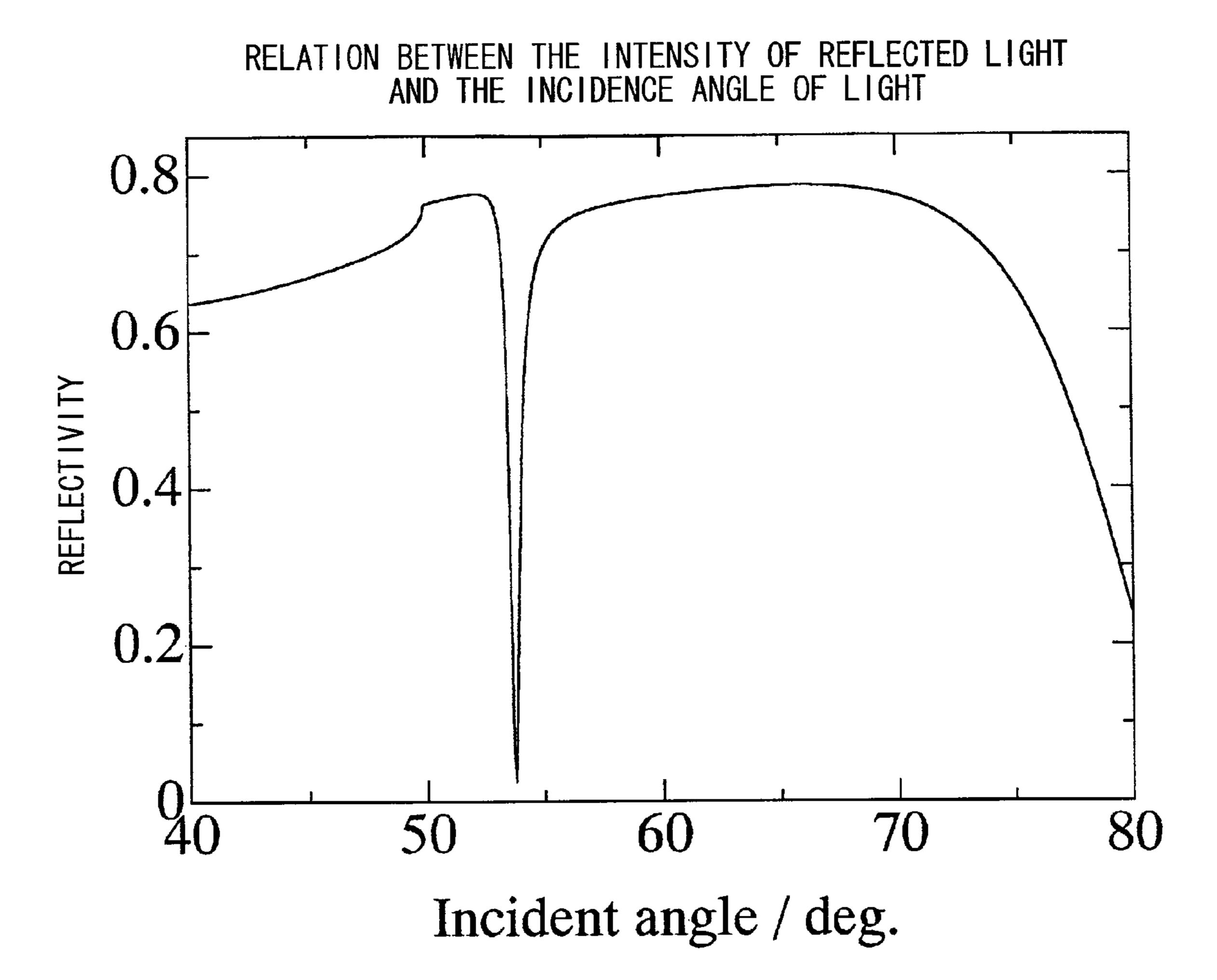
INCIDENT LIGHT: P-POLARIZED LIGHT OF 633 nm
