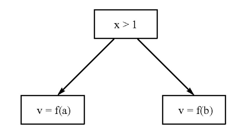
Thus, for each source code statement, code parser 208 uses the instruction logic to determine the number of nodes that CFG generator 210 generates and the connections between each node. CFG generator 210 then connects the individual
